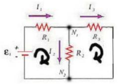
This circuit can be easily solved by reducing the two resistors,  $R_2$ , and  $R_3$ , that are in parallel, to an equivalent resistor  $R_{eq} = R_2 R_3 / R_2 + R_3$ . Then the circuit looks like
