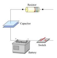
Figure 1: *RC*-circuit
