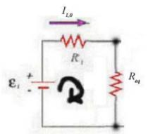
The current from the voltage source can now be easily determined,
