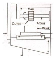
Figure 20: Horizontal Milling Machine
