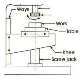
Figure 21: Vertical Milling machine
