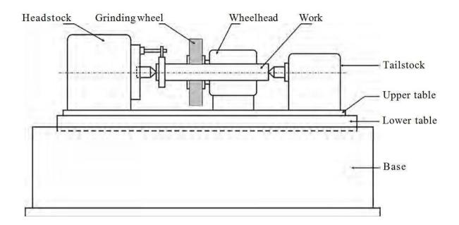
Figure 29: Cylindrical Grindin Machine
