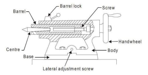
Figure 5: Tail stock of central lathe
