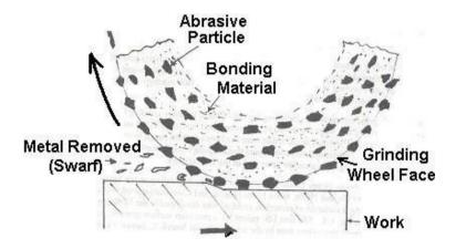
Figure 31: working principle of Grinding Wheel
