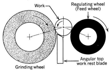
Figure 30: Centreless grinding mechanism
