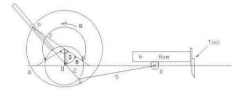
Figure 15: Whitworth - quick return mechanism
