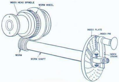
Figure 26: Simple Indexing Mechanism
