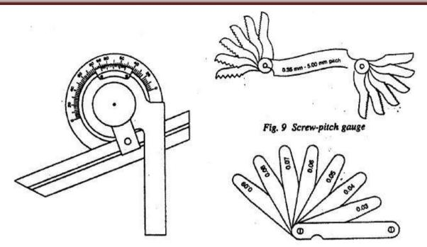
Fig. 8 Bevel Protractor
