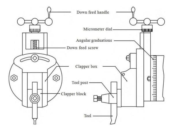
Figure 14: Shaper Tool Head
