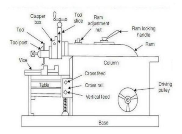
Figure 13: Standard Shaping Machine
