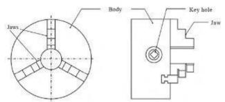
Figure 6: Three Jaw Universal Self Centering Chuck
