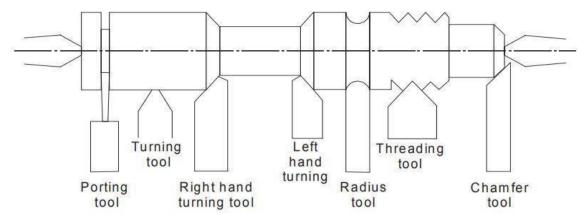
Figure 8: Various lathe operations
