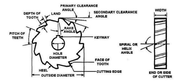
Figure 23: Nomenclature of Milling Cutter
