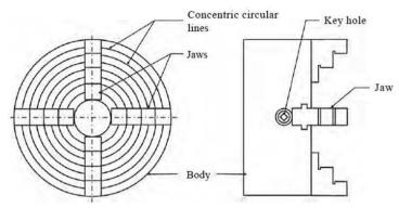
Figure 7: Four Jaw Independent Chuck
