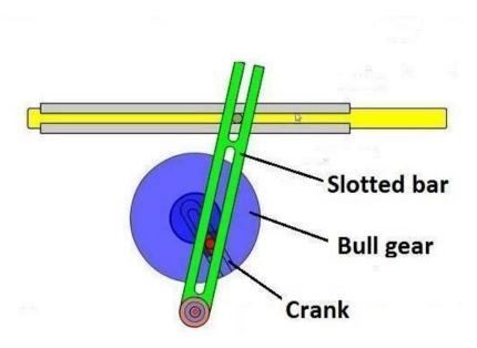
Figure 16: Crank and slotted link mechanism
