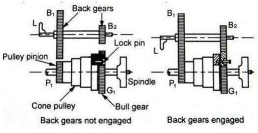
Figure 12: Back Gear Mechanism
