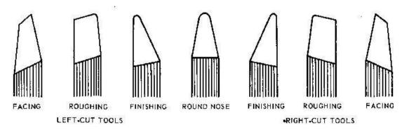
Figure 3 Standard Cutting Tools
