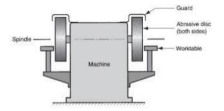
Figure 28: Bench Grinding Machine
