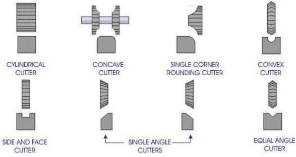
Figure 22: Different types of milling cutters
