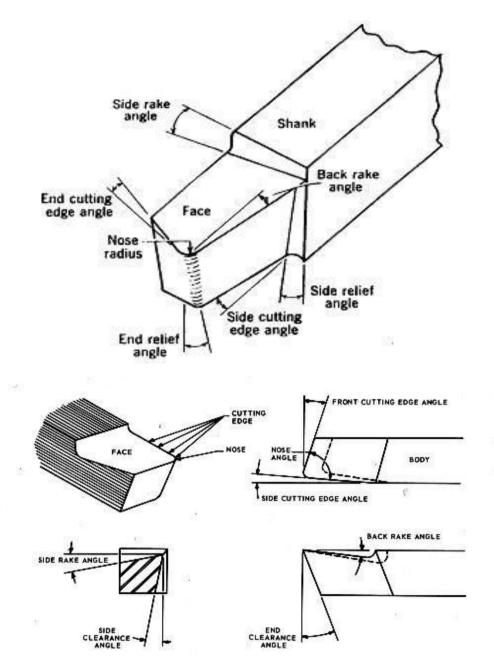
Figure 2 Cutting Tool Terminology
