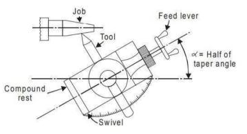
Figure 9: Taper turning by swiveling compound rest
