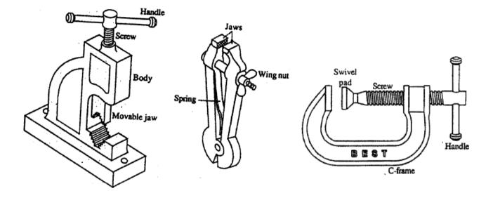
Fig. 23 pipe viseFig. 24 Hand viseFig. 25 C -clampC-clamp: C-clamp shown in fig.25 is used to hold work pieces on machines and is alsoused of clamping parts together. It consists of a cast steel frame, steel screw handle, andswivel pad. The size of the clamp is determined by the largest opening of its jaws.
