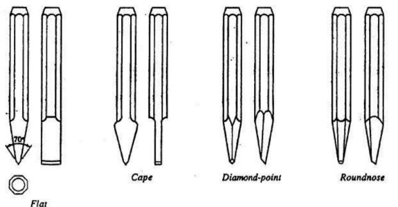
between  $50^{\circ}$  and  $70^{\circ}$  depending upon the material on which it is to be used. The cutting angle is high for hard materials and less for soft materials. It is used for chipping a considerable amount of metal from large surfaces that cannot be field or surface machined.
