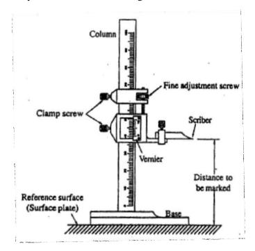
Fig. 20 Vernier height gauge
