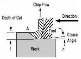
Figure 1: Basic Metal Cutting Theory against the tool.
