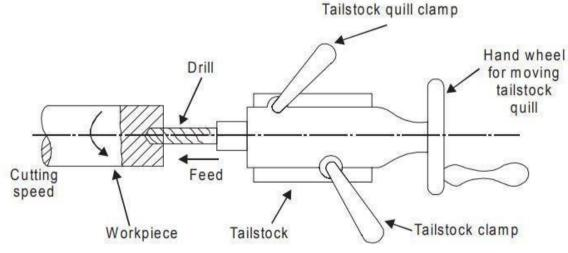
Figure 11: Drilling on lathe
