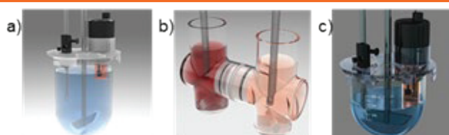
Figure 1. MacroFLUX (a) has absorption chamber (12 mL) inserted in the standard USP 1 or 2 dissolution vessel (800–1000 mL), \mu FLUX (b) uses 16–20 mL in both side-by-side dissolution and absorption chambers and BioFLUX (c) uses shortened dissolution vessel of USP 1 or 2 (200–250 mL). Note: Presented by Tsinman, K.; Borbás, E.; Tsinman, O.; Sinko, B. at the 3rd European Conference on Pharmaceutics, Bologna, Italy, March 25–26, 2019.
