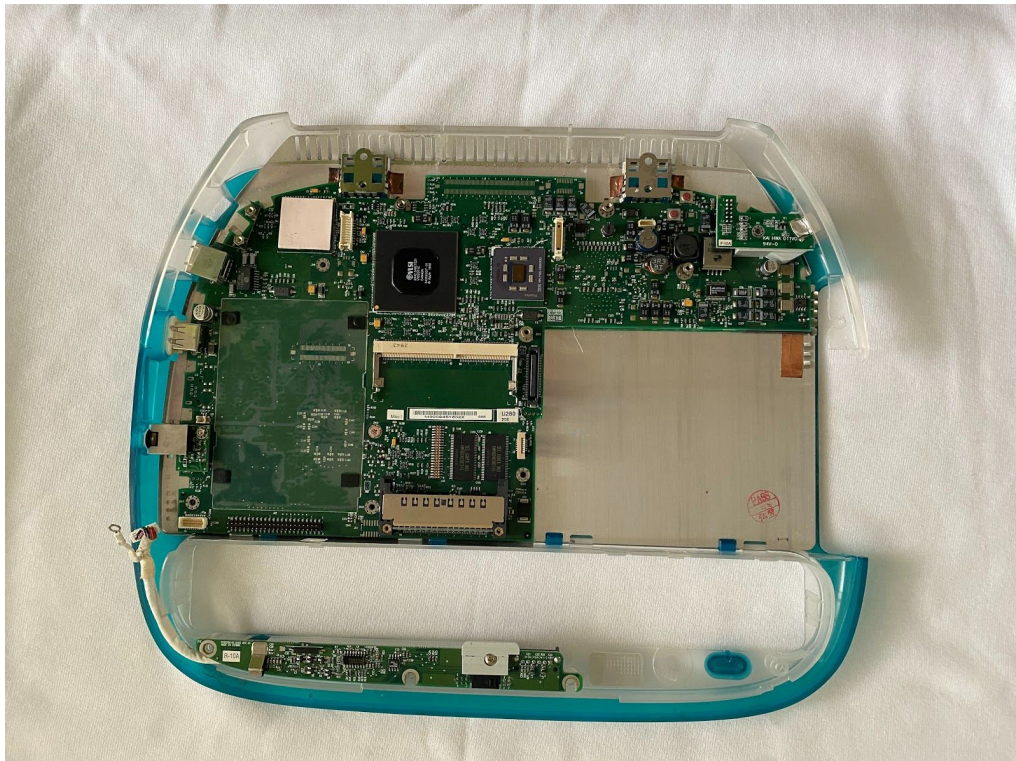
Logic Board of Clamshell, as shown attached to the bottom casing. Includes housing for CD drive, SO-DIMM memory, and modem.
