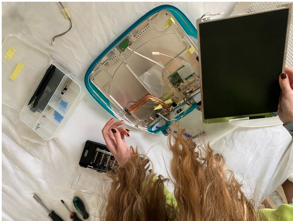
Taken while trying to disconnect the screen from copper wires and tape, LCD in the right hand. Rough 2 ½ hours into deconstruction.
