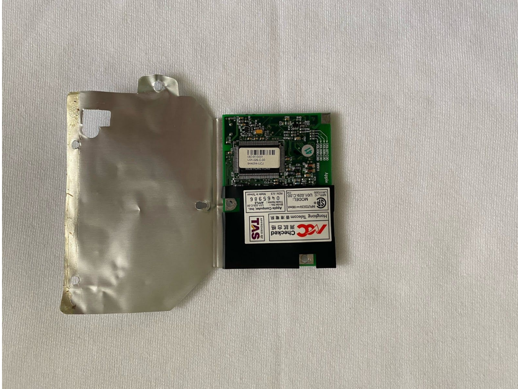
Modem found within Clamshell. Damage from prior use apparent with residue on aluminum.
