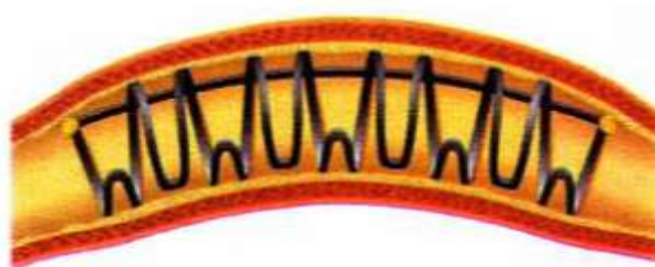
Figure 2: Cook GR11. Formed from stainless steel sheet, featuring an axial backbone with integral gold markers.
