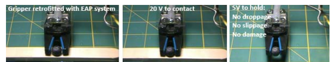
Figure 6: EMI® gripper using Synthetic Muscle™ shape-morphing system to handle a ripe blueberry with no damage.
