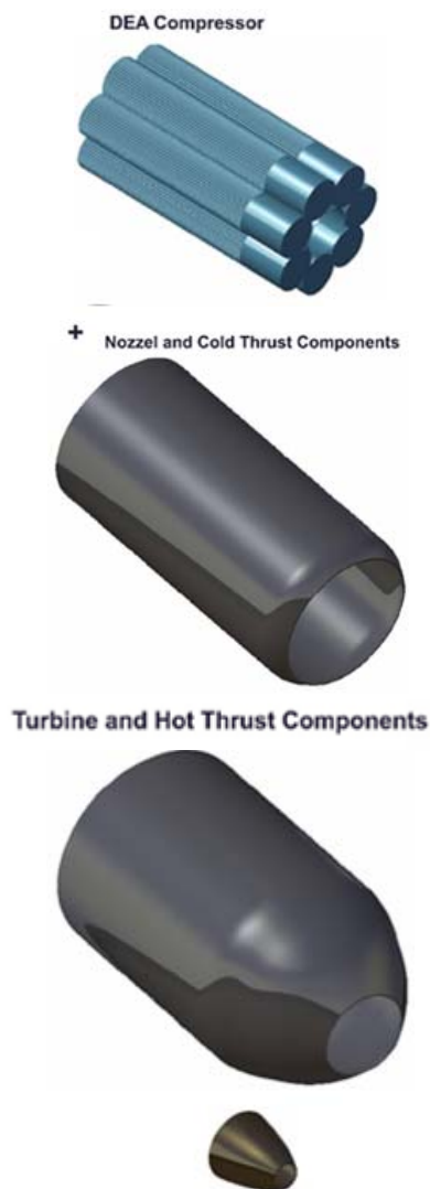
Figure 20: in a modulized engine created based on DEA compressor, a compressor unit may be used to create a PDTurboDEA or a full electric thruster. Other components define how the thruster works when compressor can operate in different configurations.
