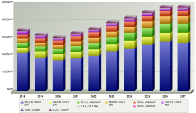
Figure 4 highlights total installed power output for the 2018–2027 period by power class. It is apparent that the 250–500 MW class is the backbone of the power generation industry and looks set to hold this position for at least the next decade.
