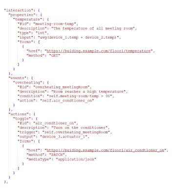
Fig. 2: Overview the WoT-AD interaction section
