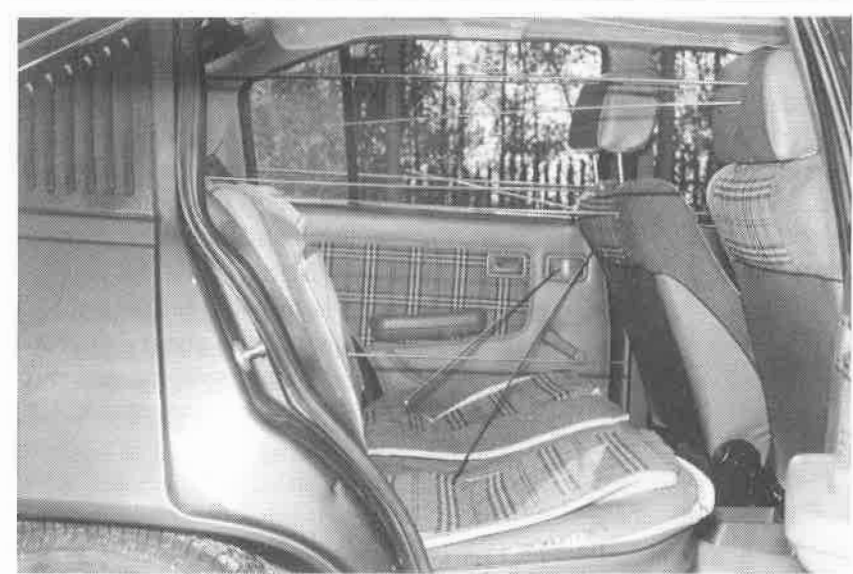
FIG 2 - Rods through hole 4 and hole 8. Hole 4 is indicated by the horizontal rod through the rear seat back. Hole 8 is indicated by the rod angling downward, backward, and left-to-right, passing through the ashtray in the left rear door.
