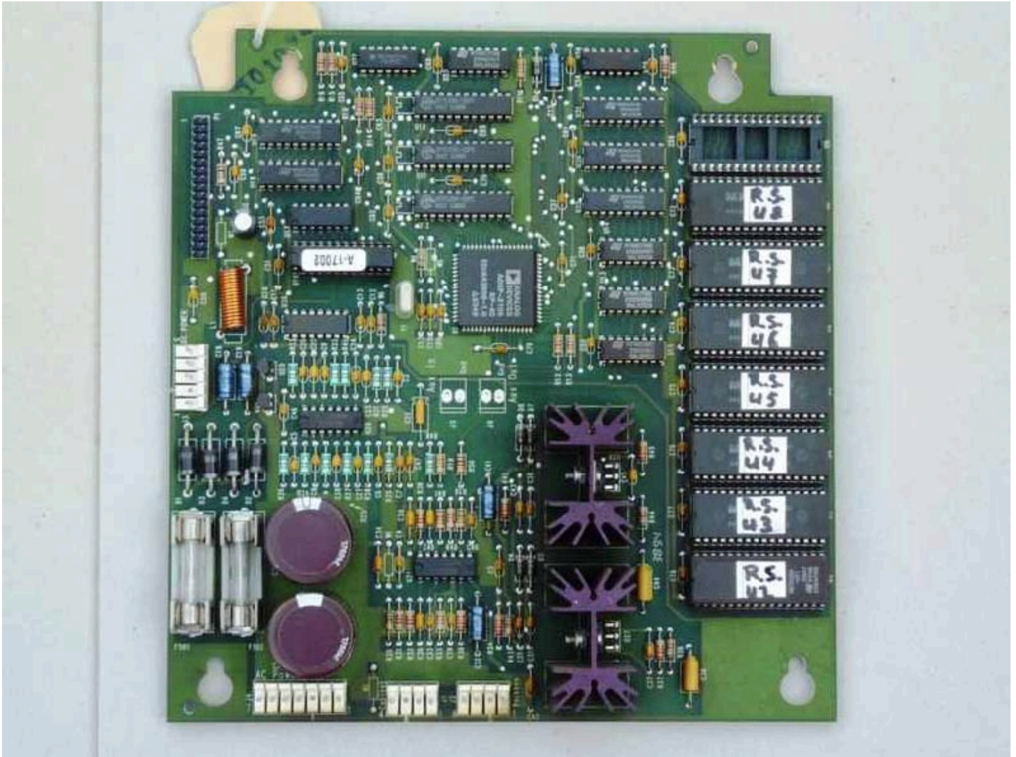
A-16917 DCS sound board. Can be recognised with all the eproms on the right.
