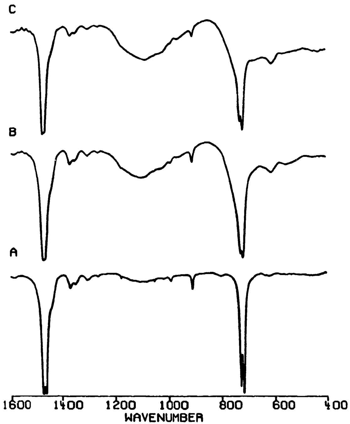
Figure 32. Mid IR of \text{Sb}_2\text{S}_4 (A) Virgin; (B) 425°C in Air; (C) 575°C in Air.
