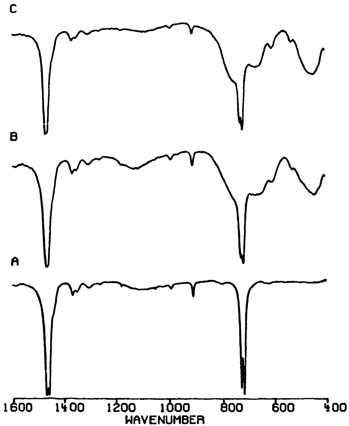
Figure 33. Mid IR of Sb_2S_4 (A) Virgin; (B) 650°C in Air; (C) 1050°C in Air.
