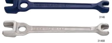
Cat. No. Description Large End Opening **Small End Opening** Color Length Weight (lbs.) 3146 29/32" and 1-3/32" 13" (330 mm) 1.85 For 5/8" hardware. 5/8" and 13/16" dark blue 3146A dark blue 13" (330 mm) 1.70 For 3/4" hardware 1-1/16" and 1-5/16' 5/8" and 7/8" 3146B 1-1/16" and 1-3/16' 11/16" and 7/8" 13" (330 mm) 1.76 Bell System Type. silver
