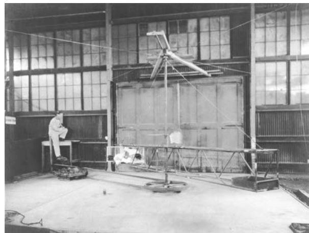
Physiological Research Laboratory centrifuge. Test subject is positioned "head-in" at the end of the rotating arm.
