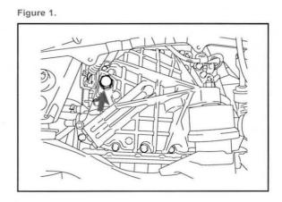
Install the Transmission Fill Adapter into the transmission fill port. SST: P/N 10002-00101-3
