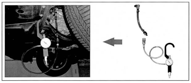
17. Attach the Fluid Extraction Tank hose quick connect to the Vacuum Regulator Manifold. SST: P/N 10002-00101-4
