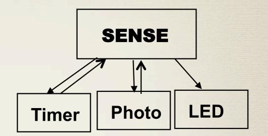
clock event handler initiates data collection sensor signals data ready event data event handler calls output command device sleeps or handles other activity while waiting conservative send/ack at component boundary
