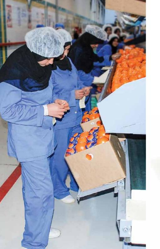
The production line goes through several stages of production such as sorting, washing, waxing and packing carried out by a group of skilled laborers who had high level of training to ensure the quality and safety of products. using various type of packing, such as telescopic cartons, open top cartons, bins and netpacking complying with high international standards.
