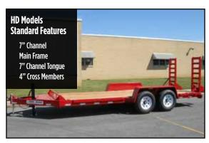
For hauling heavier equipment, skid steers, tractors and just about anything on wheels, our EH Series equipment trailers range from 10,000 GVWR to 14,000 GVWR. Carry up to 11,000 payload on our 14-HD units.
