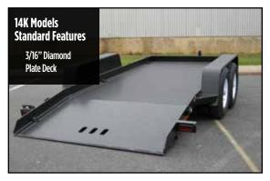
An affordable tilt trailer that saves your back. No more ramps to deal with, simply unlatch the deck and the bed tilts to the ground for a low 12 degree load angle.
