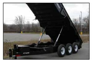
Available in 12', 14' and 16' models and built for the serious contractor, our LPHD Series dump trailers are ready for the toughest jobs. Need even more payload? Check out the 16' tri-axle model with a GVWR of 21,000#.
