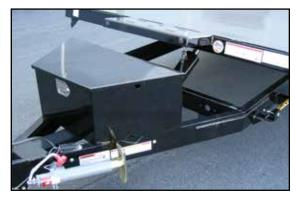
Make loading easier with our power CHT Series of tilt car haulers. Winch plate and 4 recessed D Rings along with a full diamond plate deck are standard. Remove either fender for easier vehicle access.
