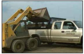
Turn your pick-up into a dump truck with our 6' or 8' dump insert. Complete with a 4" double acting hoist, this dump insert can handle over 2 tons of payload. Perfect for mulch, stone and firewood.
