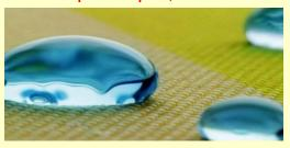
material the surface is made of. Because its design relies only on the physical attributes of the texture, the texture could have industrial or biomedical applications. For example, the surface could slow corrosion and extend the life of parts in chemical and power plants, solar cells or cookware.
