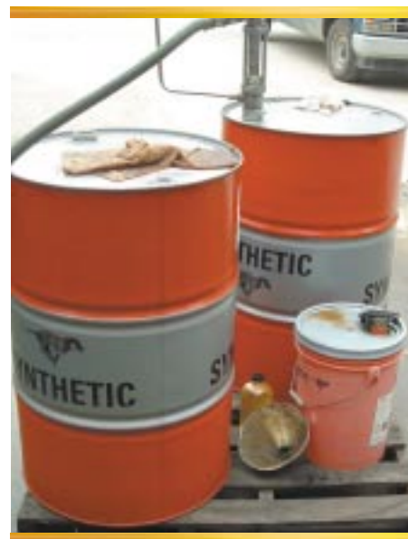
Improper fluid handling methods
