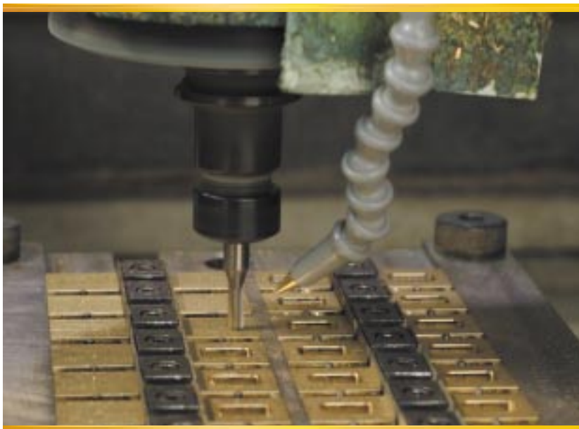
Minimum quantity lubrication used during a milling operation.
