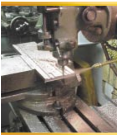
Spray cooling during milling operation.
