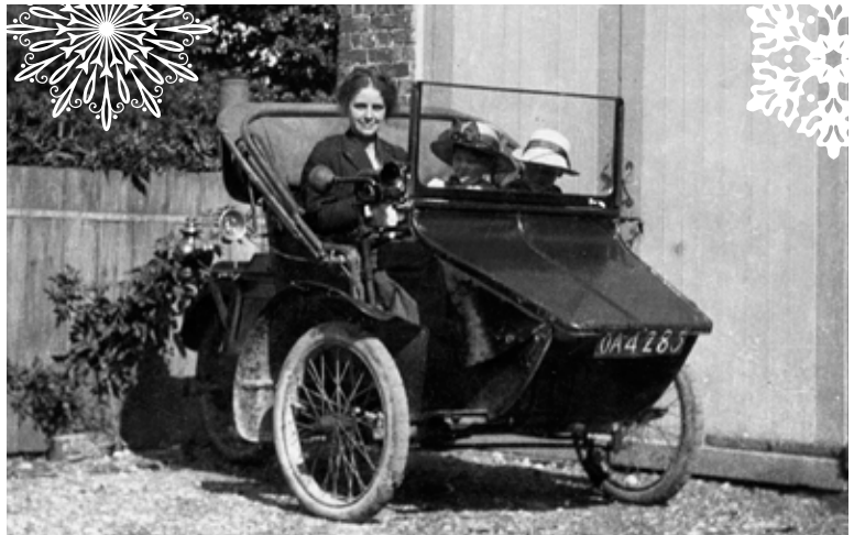
Above: in 1907 AC replaced the goods box of its Auto-Carrier delivery vehicle to create the company's first passenger car, the Sociable.
