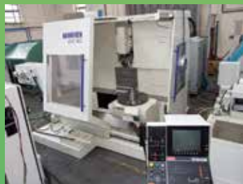
MIKRON UMC900 5 axis universal CNC milling machine, Heidenhain 426, hori / vertical spindles, probe, 5 axis, 630mm diameter table, 8000 cutting hours, ISO 40, speeds to 6300rpm, X=630 Y=900 Z=500mm £poa
