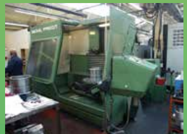
DECKEL FP5CC/T Universal CNC milling machine, 630mm dia table with C axis, Dialog 11, SK40, vertical and horizontal spindles, speeds to 6300rpm, X=800 Y=600 Z=550mm £poa
