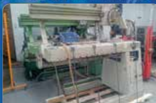
BODE 2/HSW 6/48 LONGITUDINAL SEAM WELDER Capacity 1200mm Min Diameter 150mm
