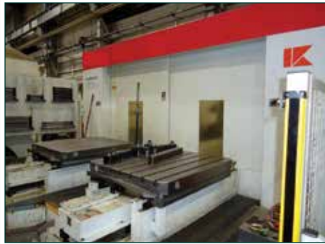
KURAKI KBM 11X-P Twin Pallet 5 Axis Horizontal Boring & Milling Machine with Fanuc 16i-MB Control. Year 2003. Spindle dia. 110mm. Spindle speeds 5 – 3000 rpm. Spindle taper SK50. X/Y/Z/W 1500mm/1000mm/700 mm/350mm. Full B Axis indexing to 0.001°. Rapids X/Y/Z 12m/min. Rapids W 6m/min. 60 ATC. Table loading 2,200kgs. Main spindle drive (AC) 18kW. Fully enclosed photo-electronic interlocking guarding. Swarf conveyor. Filtermist unit. High pressure coolant. Through spindle coolant. Spindle cooling unit. Twin Pallet Shuttle System.
