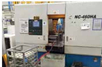
Everising NC-460 HA fully automatic Bandsaw (2006)
