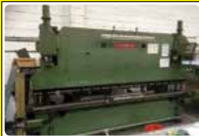
PEARSON 10012 3.7m x 100ton hyd pressbrake, guards
