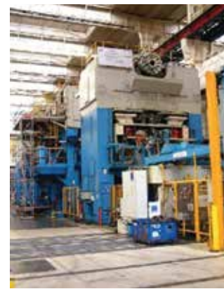
Stock-No. 1050-153061A Screw Press WEINGARTEN PA 225 Year of manufacture 2008
