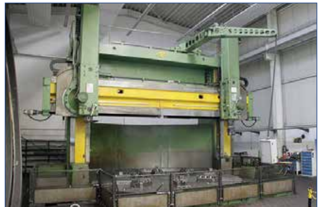
STANKO 1563 CNC VERTICAL BORER WITH SIEMENS 840D 5 axes CNC controlled, with C-axes 360.000 degrees for positioning, one CNC-Support with live spindle, 28 kW, cooling through spindle, one CNC-support for turning. Table diam. 6300 mm. Max swing 6.500 mm. Working height 3.200 mm. Table load 160 tons. Main Motor 125 kW. Machine installed unused and modernized 2004-5.
