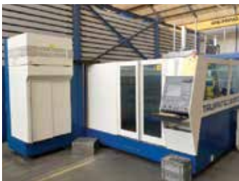
Manufacturer: Trumpf Type: Trumatic L6050, 6kW Year: 2006 Control: Siemens Sinumerik 840 D
