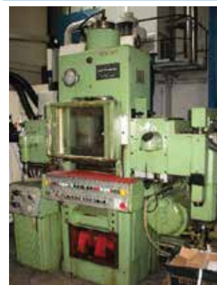
Stock-No. 1050-113044 Fine Blanking Press FEINTOOL GKP-F 50/80 Year of manufacture 1971
