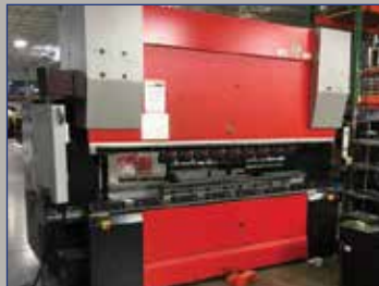
146 TON X 123" AMADA HFE 1303 M2 "DOWN-ACTING" CNC PRESS BRAKE. MFG: 2010. STOCK NUMBER: 10435
