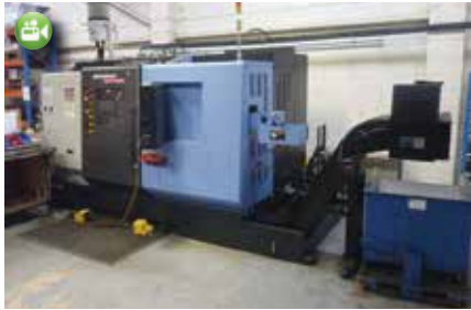
Doosan Puma TT1800SY (2011) Fanuc 31i Control
