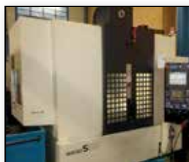
VERTICAL CENTER MAKINO S56 YEAR 2007 HSK SPINDLE 20000RPM TRAVELS 900X500X450MM 30ATC
