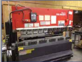
88 TON X 98" AMADA RG-8024LD "UPACTING" HYDRAULIC PRESS BRAKE. MFG: 1999. STOCK NUMBER: 10425
