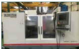
CININNATI Arrow 750 Vertical Machining Centre with Acramatic Control. Year 2003. Table size 950mm x 520mm. XYZ travels 762mm/510mm/510mm. Feeds 0-12m/min. Rapids 20m/min. Spindle speeds 60-8,000 rpm. 30 ATC.
