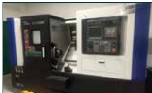
HYUNDAI Wia L230LMSA Slant Bed CNC Lathe with C Axis & Driven Tooling Fanuc 32i. Year 2014. Main spindle Chuck dia. 210mm. Maximum swing 55 mm. Turning dia. 309mm. Turning length 520mm. Spindle bore 77.97mm Bar capacity 66mm. Main spindle 4,000 rpm. Main spindle nose A2-6. 20HP. Sub spindle nose A2-5.
