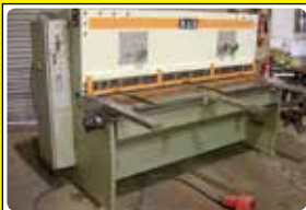
K & B 2m x 4mm hyd shear, PBG, BGA, Vari-rake
