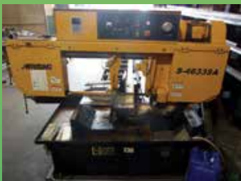
EVERISING S4633 SA Semi Automatic Horizontal Bandsawing Machine, New 2007, Bidirectional angle adj -60° ~ 0° ~ +45° Bi- Direction, coolant, hydraulic flow down feed control, 330mm max dia saw £poa
