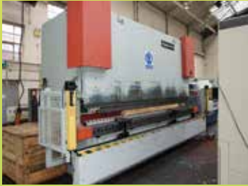
EDWARDS PEARSON RT4 330 x 4100 CNC press brake, Cybelec DNC 90 Colour 3D CNC, tooling, light guards, 265mm stroke, 3750mm between frames, 330tons x 4100mm capacity £poa
