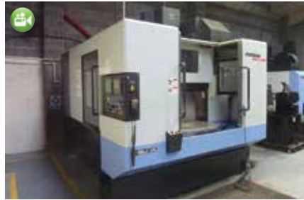
Doosan Ace VC500 (2009) Fanuc 21i Control + Kitagawa 4th Axis
