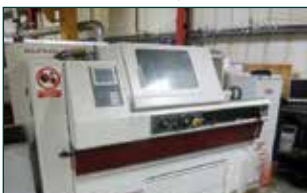
HARRISON Alpha 330T CNC Lathe with GE Fanuc Control. Year 2004. Swing over bed 330mm. Swing over cross slide 210mm. Distance between centres 100mm. Spindle speeds 0-3500 rpm. Year 2003. Table size 840mm x 420mm. Main motor 7.5 kW Spindle capacity 40mm. GE Fanuc Quick Panel Control. Fitted with 3 jaw chuck Quick change toolpost with toolholders.
