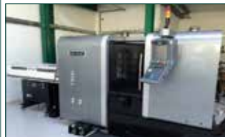
HURCO TM8i CNC Lathe with Hydrafeed MV65 Barfeed. MAX CNC Control. Year 2013. Max. cutting diameter 250 mm. Max. cutting length 450 mm. Chuck diameter 203 mm. Bar Capacity 52mm. X-Axis 203 mm. Z-Axis 508mm. Feeds XYZ 19/24 mm. Spindle-motor 16 kW. Torque 180 Nm. Spindle speed 0-4800 rpm. 12 station turret VDI30.
