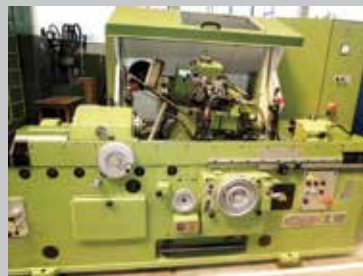
REISHAUER Universal Thread- & Worm-Grinder UL 900 yr. 1990 Ø 250 x 900 mm, relieve grinding attachment
