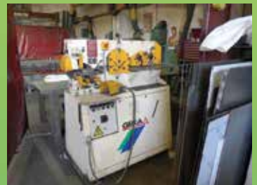
GEKA MINICROP universal steelworker, Selection of punches and dies, four work stations, foot control, 27mm dia x 13mm max punch, 300 x 10mm shearing £poa
