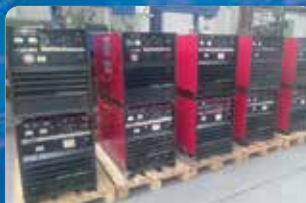
LINCOLN DC 1000 AMP WELDING POWER SOURCE SUPPLY Heavy Duty for MIG, Flux-Cored, SAW and Gouging
