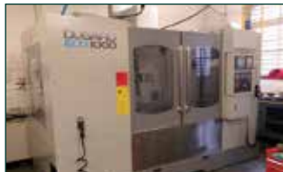
DUGARD ECO 1000 Vertical Machining Centre with Fanuc 0i-MD Control. Year 2012. Table size 1300mm x 600mm. XYZ travels: 1000mm/600mm/600mm. Spindle motor 11/15kW. Spindle speeds to 8,000 rpm. Spindle taper BT40. Thro. spindle coolant. Footprint 5230mm x 3295mm. Weight 5,000 kgs.
