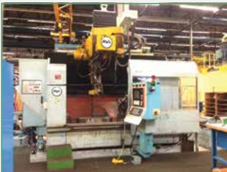
BERTHIEZ RVR 100 CNC Rotary table vertical grinder
