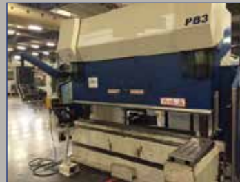
257 TON X 127" TRUMPF TRUMABEND V230 CNC PRESS BRAKE. 6-AXIS CNC BACKGAUGE. CROWNING. UPPER & LOWER HYDRAULIC CLAMPING. MFG: 2004. STOCK NUMBER: 10404
