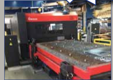
4000 WATT AMADA FO3015MII RI LASER CUTTING SYSTEM WITH ROTARY INDEX. MFG: 2012. STOCK NUMBER: 10320
