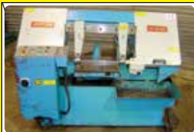
BIGSTONE CF-350M semi-auto mitre bandsaw, 280mm dia
