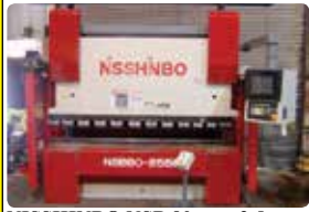
NISSHINBO NSB 80ton x 2.5m CNC pressbrake, 7 axis
