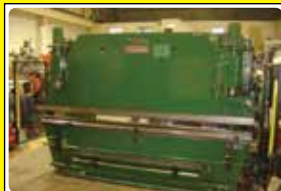
PEARSON 7010 3m x 70ton hyd pressbrake, tools, guards
