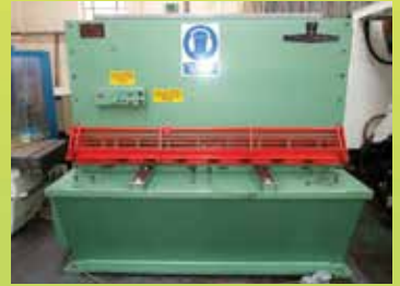
ELGA HYDRASHEAR 612 Hydraulic guillotine, Squaring arm, front supports, blade gap adj, power back gauge, finger guards, Hydraulic, 2050 x 13mm capacity £poa
