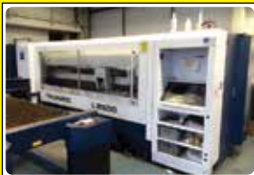
TRUMPF TRUMATIC L2530 CNC Laser, 1.25 x 2.5m, 3.2kw
