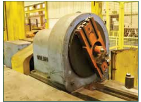
WALDRICH Roll Grinder. Swing 1,220mm x 6,500mm Between Centres with Cambering and DRO. Swing over bed 1,220mm. Distance between centres 6,500mm. Wheel dia. 711mm x 304mm & 355mm bore. 2off Steadies 88mm – 355mm dia. (with extensions) 2 off Steadies 355mm – 610mm. Cambering system. Coolant/Magnetic filtration unit. Total weight 30,000kgs approx.
