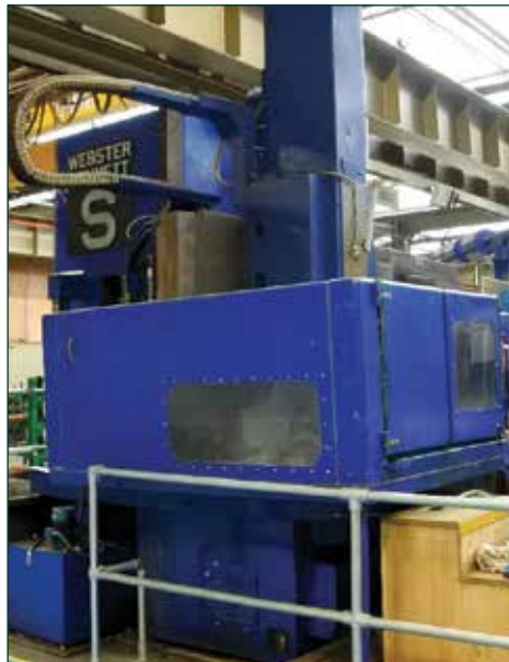
WEBSTER & BENNETT Series S Elevating Rail Ram Type CNC Vertical Borer with Philips 3000 Control. Table dia. 1000mm. Maximum swing 1750mm. Height under cross rail 1600mm. Maximum height under ram 1854mm. Ram section 203mm x 203mm. Vertical travel of ram 1219mm. Speeds 12 – 324 rpm (inf.var). Table loading 10 Tons. Elevating Rail. Ram type. Auto tool changer. Chuck jaws. Philips 3000 Control. Main motor 75 HP. Year 1981. Total weight 17,400kgs.
