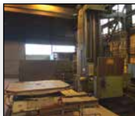
FLOOR TYPE BORING SCHIESS FRORIEP SPD 150MM DIGITAL TRAVELS 7000X3700MM SKODA TABLE 2000X2000MM
