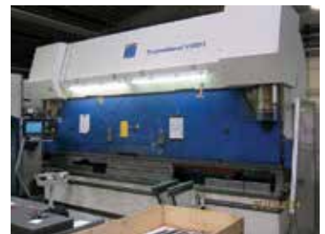
Manufacturer: Trumpf Type: TrumaBend V 320 Year: 2000 Press force: 320 to
