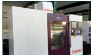
BRIDGEPORT VMC500-16 Vertical Machining Centre with GE Fanuc 18-M Control. Year 1998. Table size 837mm x 358mm. XYZ travels 500mm/340mm/520mm. Spindle Speeds 40 - 8000 rpm. Spindle taper BT40. Spindle Motor Power 7.5kW. 16 position auto toolchanger. Coolant. Interlocked guards. Low Volt Light. Ex Training School.
