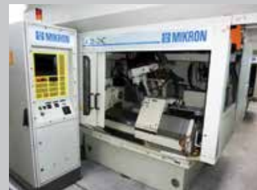
MIKRON CNC-Gear Hobber A 35/36 Ø 200 x Mod 4 x 300 mm with workpiece loading
