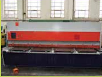
BYSTRONIC BYSHEAR VR6.5/4100 CNC guillotine, New 2008, Cybelec CNC, rear sheet support, squaring arm, supports, rear light guards, 4100 x 6.5mm capacity £poa
