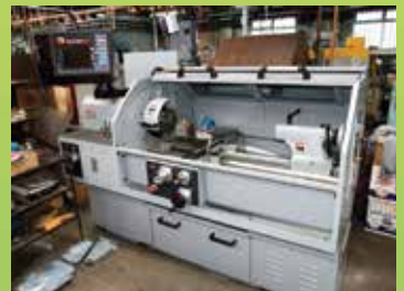
XYZ SLX355 CNC Lathe, New 2012, 360mm swing over bed, 1000mm between centres, 52mm spindle bore, Prototrak SLX CNC, speeds to 4000rpm, 100 hours use £poa
