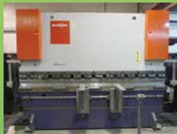
BYSTRONIC AFM EP 100/3100 CNC press brake, New 2005, well tooled, Cybelec DNC 880, front supports CNC crowning, Lazer guards, 200mm stroke, 100ton x 3150mm capacity £poa
