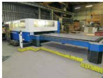
Manufacturer: Trumpf Type: Trumatic L4030, 2,7kW Year: 2003 Control: Siemens Sinumerik 840 D
