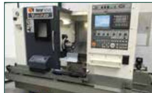
VICTOR Vturn P20 CNC Slant Bed Lathe with Fanuc 0i-TD Control. Year 2014. Swing over bed 520mm. Max turning dia. 260mm. Distance between centres 440mm. Spindle speeds 4200rpm X travel 20mm + 140mm. Z travel 370mm. Rapids 30m/min. Spindle bore 66mm. Fanuc 0i-TD Control with 10.4" Graphic Display. 10 Station Turret with Toolholders.
