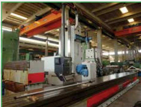
ZAYER 30 KMU 14000 CNC Bed milling machine
