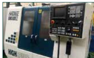
HARDINGE VMC 600 II High Speed Vertical Machining Centre with Fanuc 18-M Control. Year 2001. Table 750mm x 355mm. XYZ travels 600mm/500mm/508mm ATC 20. TSS27 Tool Probe. Spindle Taper BT40. Spindle Speeds 8,000 rpm. Fanuc 18-M Control. Dimensions 2133mm x 2463mm x 2565mm high. Weight 4400 kgs.
