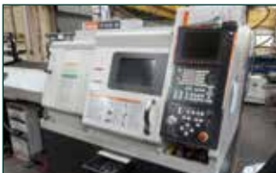
MAZAK Nexus Quick Turn 100 with Mazatrol 640 Fusion Control. Year 2005. Swing over bed 540mm. Swing over cross slide 270mm. Max turning length 307mm. Max turning dia. 275mm. Spindle speeds to 6000rpm. Spindle bore 60.9mm. Bar capacity 41.27mm. 12 station turret. Complete with collet chuck, Paris catcher.
