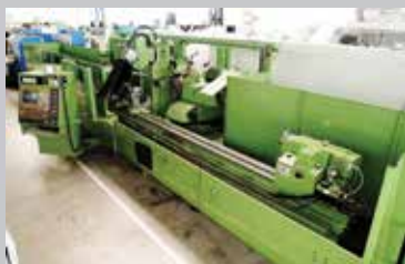
GLEASON-PFAUTER CNC-Gear-Profile Grinder P 1200 G yr. 2007 Ø 1200, SIEMENS 840 D, with measuring
