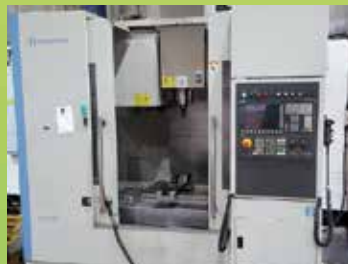
HARDINGE BRIDGEPORT GX 600 vertical machining centre, New 2011, 4th axis, handwheel, speeds to 10000rpm, Siemens 828D, BT40, 750 x 540mm table, X=600 Y=540 Z=430mm £poa
