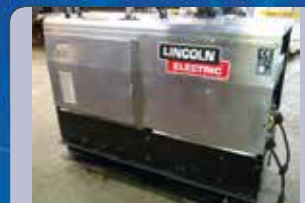
LINCOLN VANTAGE 500 DIESEL WELDER GENERATOR POWER SOURCE with Perkins Engine
