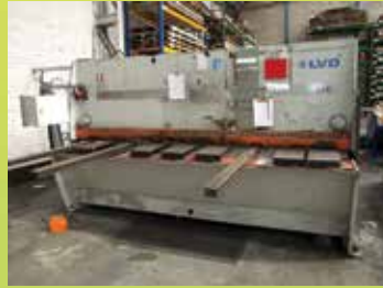
LVD MVS-TS 31/6 CNC Guillotine, New 2005, LVD CNC touch screen, sheet support system, blade gap, vari rake, light guards, 3100 x 6.5mm capacity £poa
