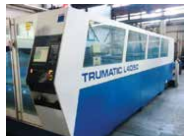
Manufacturer: Trumpf Type: Trumatic L4050, 6kW Year: 2004 Control: Siemens Sinumerik 840 D
