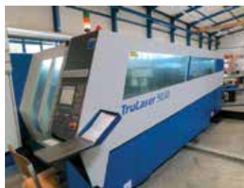
Manufacturer: Trumpf Type: TruLaser L5030, 6kW Year: 2008 Control: Siemens Sinumerik 840 D
