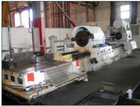
WOHLENBERG B800P Heavy Duty Deep Hole Borer & Trepanning Machine. This machine is a "P" Version. The "P" version is suitable for boring heavy, asymmetrical or awkwardly shaped workpieces, which cannot rotate. Workpieces of this type are clamped to a T slotted indexing work table which has the capability of indexing 360 degrees in 4 x 90 degree graduations. The tool headstock drives the boring tool. Boring feed is produced by the boring carriage. Spindle drive 100 HP. Spindle speeds 85-1120 rpm. Table size 60" x 60" (1524mm x 1524mm).
