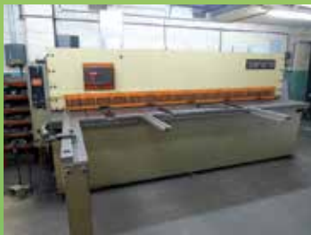
SAFAN VS 310-6 hydraulic guillotine, Digital backgauge, squaring arm, support arms, blade adj, foot control, 3100 x 6mm capacity £poa
