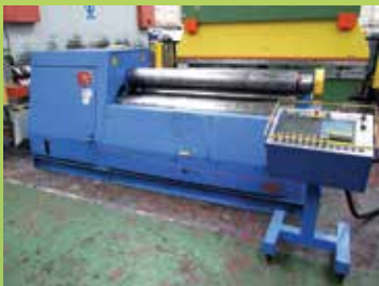
MG EH216C CNC 4 roll bending rolls, New 2002, CNC controlled, cone rolling, hydraulic drop end, top roll dia 270mm, double pinch, pre bend 14mm, 2050 x 16mm capacity £poa
