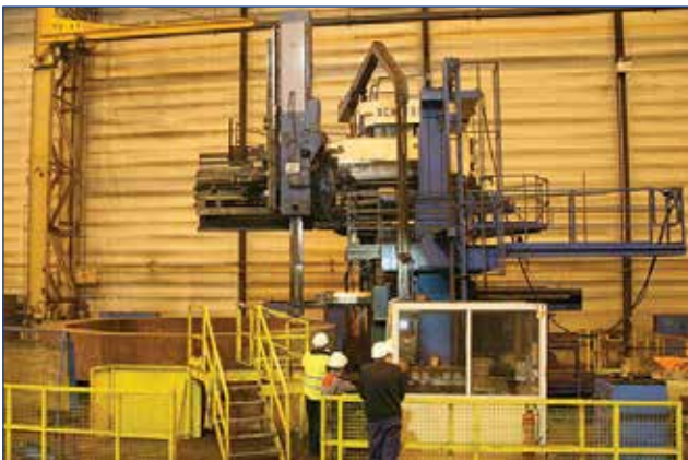
VERTICAL BORER SCHIESS 3/2 VKE 420/900 Diam 9000 mm! Table diam 4.200 mm, Max. Swing 9.000 mm, Table load 90 Tons. Max. Turning height 3.600 mm.
