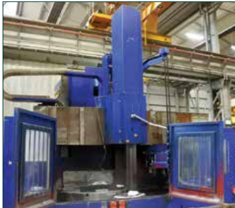
WEBSTER & BENNETT Series S Elevating Rail Ram Type CNC Vertical Borer. Fanuc 18i-T Control. Year 1981. Table dia. 1270mm. Maximum swing 1750mm. Height under cross rail 1600mm. Maximum height under ram 1854mm. Ram section 203mm x 203mm. Vertical travel of ram 1219mm. Speeds 12 – 324 rpm (inf.var). Table loading 10 Tons. Elevating Rail. Ram type. Auto tool changer. Chuck jaws. Fanuc 18i-T Control. Main motor 75 HP. Total weight 17,400kgs.
