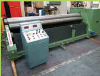
SERTOM 3002 4R hydraulic bending rolls, 4 roll double pinch, mobile control with 2 LED read outs, 250mm dia top and bottom rolls, 3050 x 8mm capacity £poa
