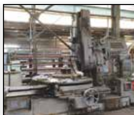
GEAR SHAPER MAAG SH 180/300 CAP 3,000MM
