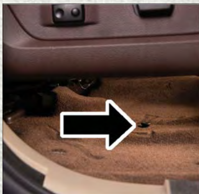
Floor Fastener Location
