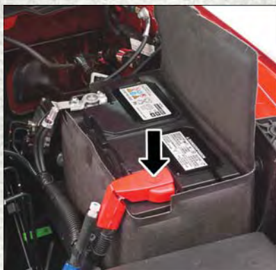
Battery Positive Post
