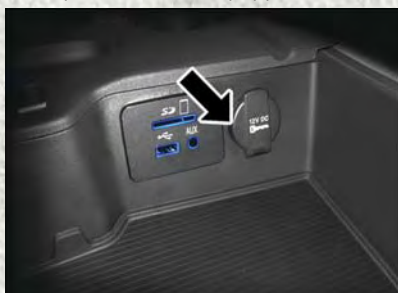
Power Outlet — Storage Compartment
