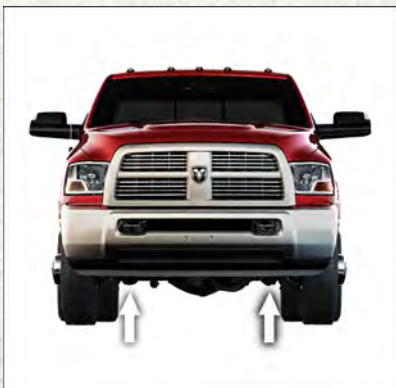
Front Jacking Location
