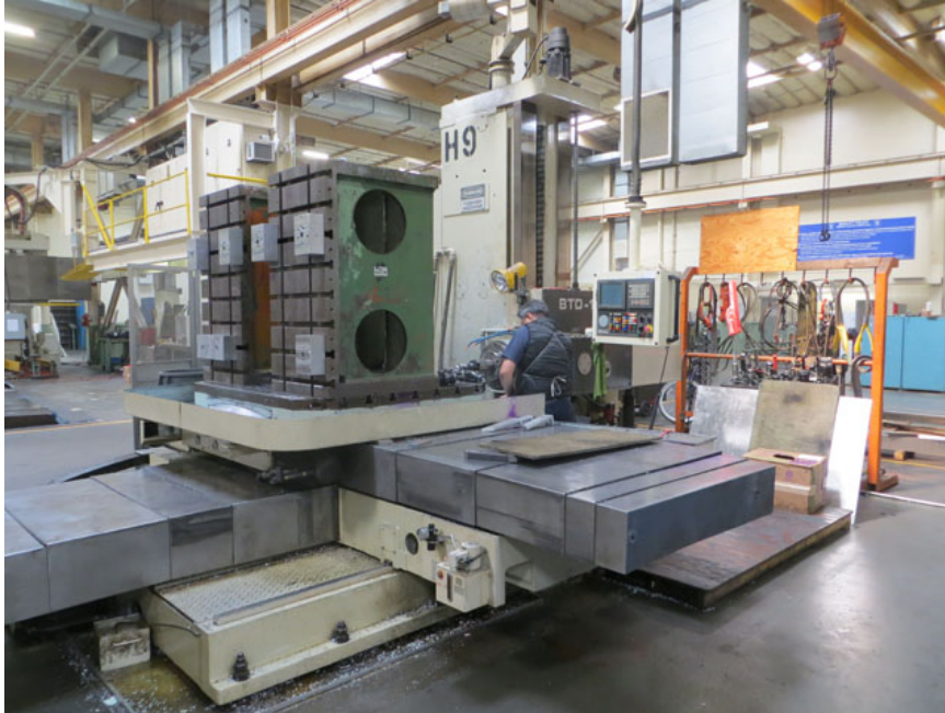
(H-9) Toshiba 4" Spindle X = 78", Y = 52", Z = 51", W = 24" Fully Programmable 55"X63" Rotary Table
