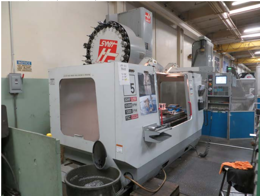
(H-12) Haas Model # VF5 30 HP X = 50", Y = 26", Z = 28" 10,000 RPM
