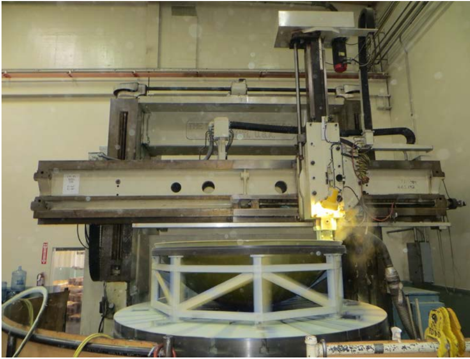
(V-5) King CNC Controlled 120" Swing, 96" Under Rail
