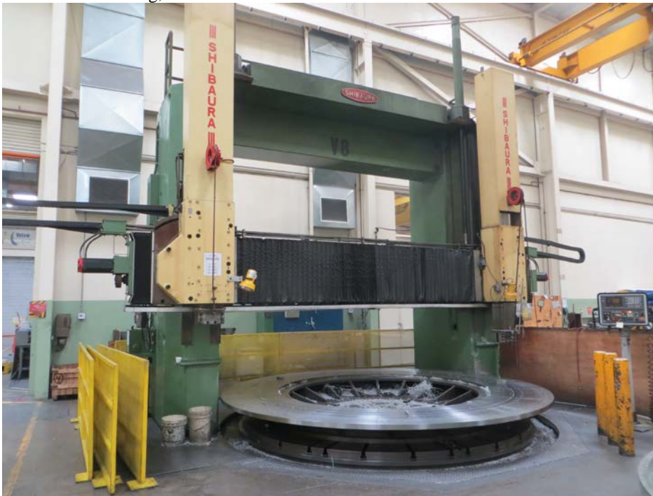
(V-8) Shibaura CNC Controlled 180" Swing, 130" Under Rail
