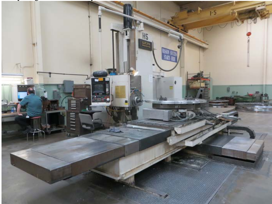
(H-5) Lucas 5' Spindle X = 106", Y = 72", Z = 38", W = 48" Fully Programmable Rotary Table
