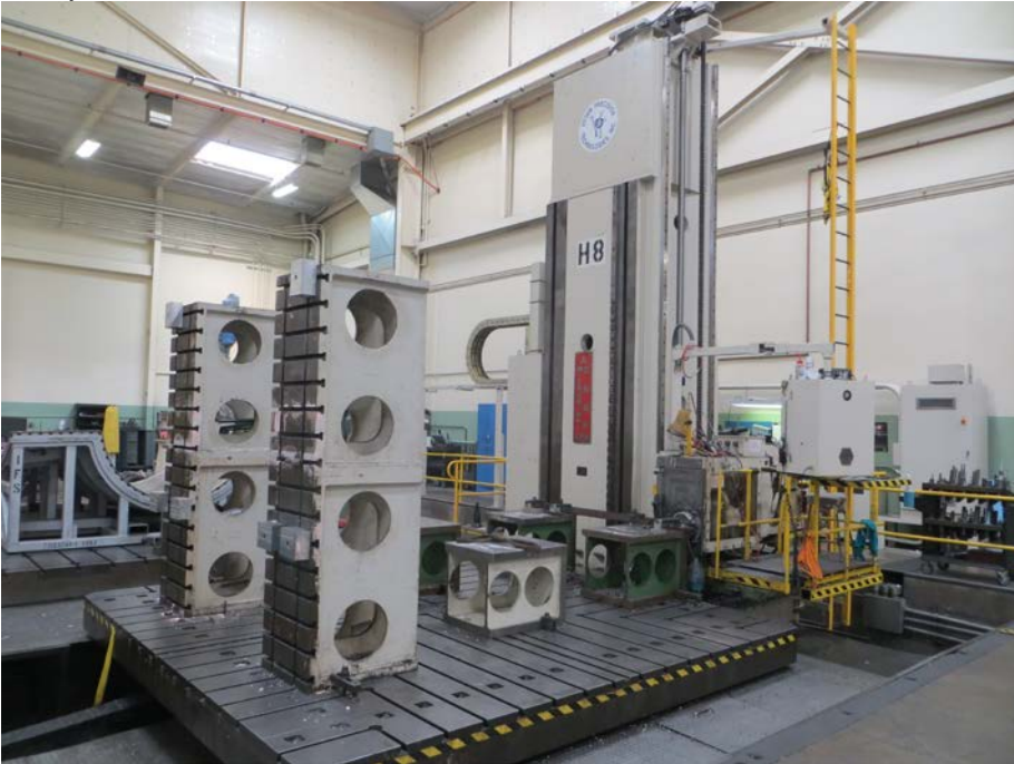
(H-8) Mitsubishi 4" Spindle, Floor Type X = 348", Y = 117", Z = 45", W = 103" Rotary Table 168" x 168"
