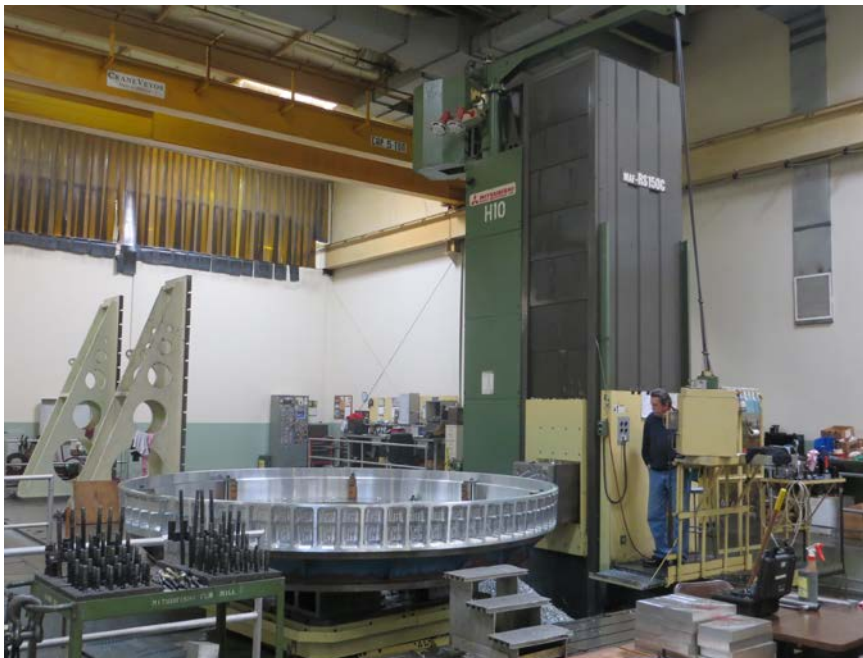
(H-10) Mitsubishi 8" Spindle Floor- Type X = 472", Y = 136", Z = 43", W = 36" Fully Programmable 86"X86" Rotary Table with an IN and OUT travel of 86"
