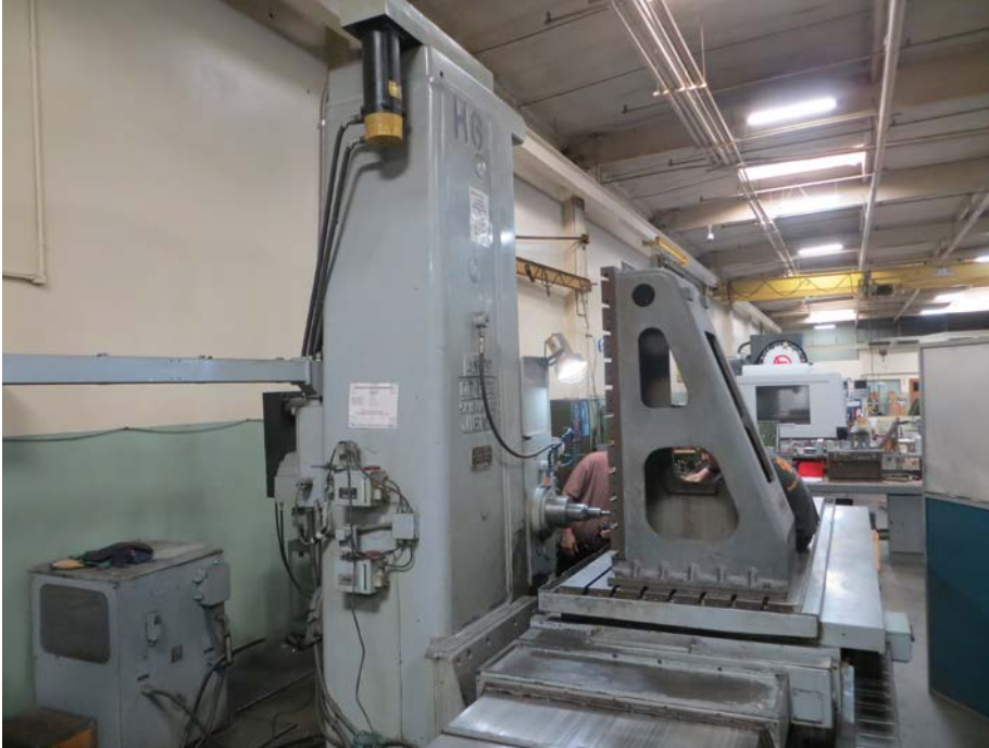
(H-6) DeVlieg 4" Spindle X = 120", Y = 72", Z = 20", W = 20"
