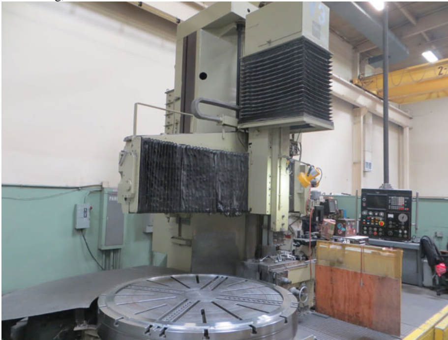
(V-3) Shibauro CNC Controlled 163" swing, 94" Under Rail
