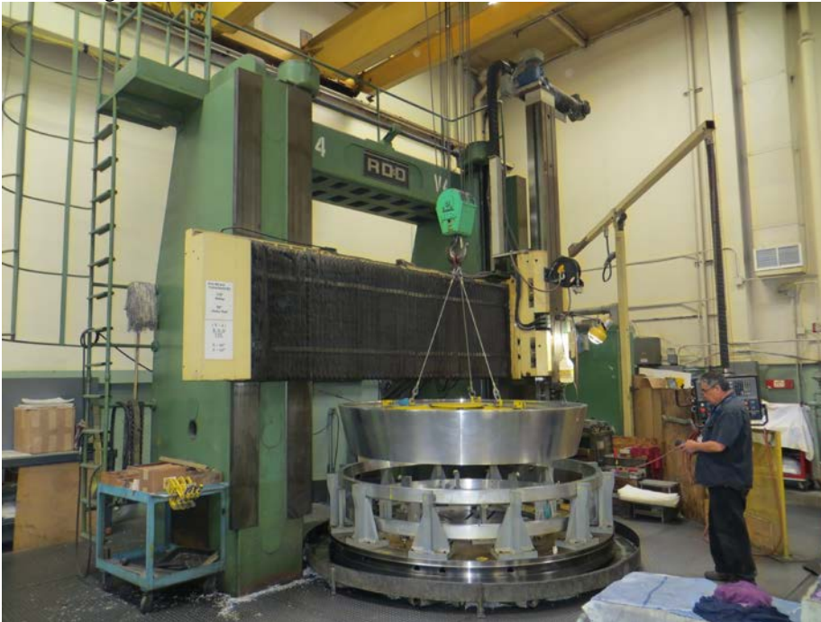
(V-4) RD & D CNC Controlled 116" Swing, 90" Under Rail
