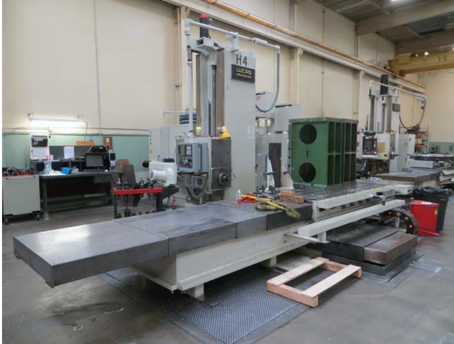
(H-5) Lucas 5' Spindle X = 106", Y = 72", Z = 38", W = 48" Fully Programmable Rotary Table
