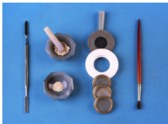
Fig. 6 Large amounts of samples, prepared for the Bragg-Brentano diffractometer.
