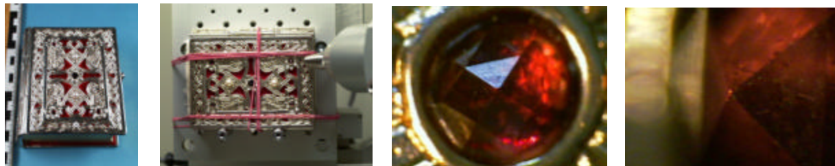
Fig. 25 Silver book cover of the bible's reprint with 5 red jewels, adjustment of the book cover to the XYZ-stage, video image and adjustment of the jewel with the laser spot.
