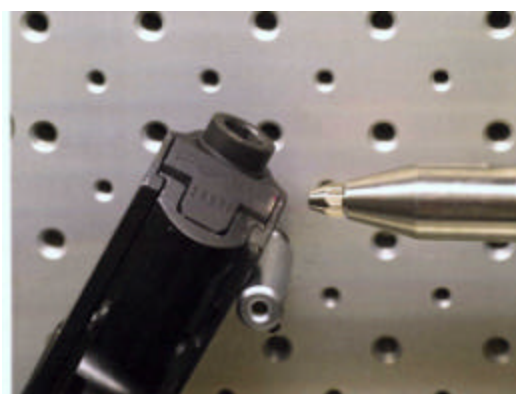
Fig. 30 Pistol mounted on the XYZ stage, contact trace specimen on the muzzle of the barrel
