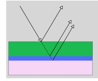
Interference of x-rays reflected from different interfaces  $\rightarrow$  several phase shifts  $\rightarrow$  beating pattern
