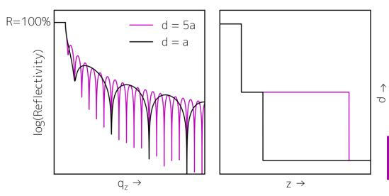
Single layer: Phase shift  $R = \frac{r_{0,1}^2 + r_{1,2}^2 + 2r_{0,1}r_{1,2}}{1 + r_{0,1}^2 r_{1,2}^2 + 2r_{0,1}r_{1,2}} \frac{\cos 2k_{z1}h}{\cos 2k_{z1}h}$
