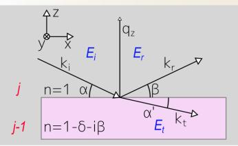
Specularly reflected intensity fraction  $R(\alpha) = \frac{I(\alpha)}{I_0}$  at  $\alpha = \beta$
