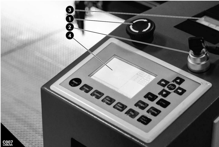
Figure C008: CO2 Laser control panel. (1) Emergency Stop. (2) On/Off Button or Key Start. (3) Ammeter. (4) Ruida Control Panel.
