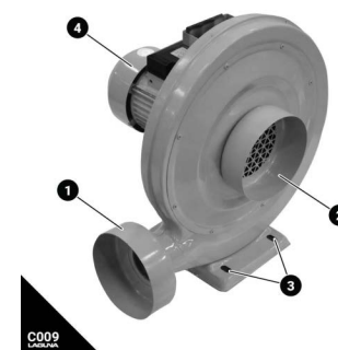
Fig C010: Exhaust Blowing unit for laser machines. (1) Positive Pressure output (air comes out here). (2) Negative pressure input (air is sucked in here). (3) Mounting Bolt Holes. (4) TEFC AC Induction Motor.
