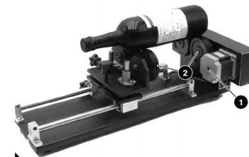
Fig C014: Rotary attachment accessories for Ruida Controlled CO2 Lasers. (1) Drive motor connected to RUIDA controller. (2) Work piece rests and rotary mechanism.
