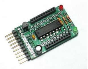
Or you can solder the header flat against the back of the adapter, so that it sticks out along the edge.
