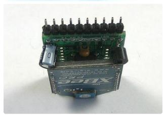
Once the electrolytic capacitor is in place, insert the 3.3V regulator and the smaller ceramic capacitor as well. The small ceramic capacitor helps filter out high frequency noise from the power supply and the regulator turns the 5V input into a nice & steady 3.3V that the XBee requires.
