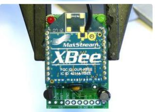
Next are the two 10-pin 2mm headers. These header sockets hold the XBee radio module securely so that it can be easily replaced or reused. Put the sockets in the two strips of holes.
