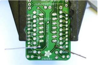
Turn the PCB over. Using your soldering iron tip, press and heat both the pad (the silver ring around the hole) and lead (wire) at the same time for 2 or 3 seconds. Then poke the end of the solder in to create a nice solder joint. Do this for both leads.
