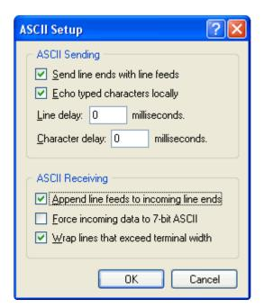
Now type in +++ (three plus signs) in quick succession. If the XBee is connected up properly you will get an OK in response.
