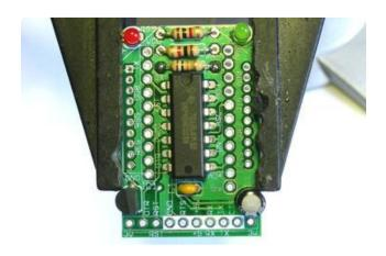
Next is the buffer chip. This chip converts the 2V-5V signal from the bottom strip of pins to 3.3V so that you can safely connect the XBee to 5V logic circuitry. If you're planning to use the two lines of parallel breakout pins instead of the lines at the bottom of the PCB, you may want to skip the buffer. However, most people will want it in place.
