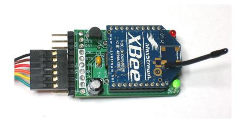
You'll need to figure out which serial port (COM) you are using. Plug in the FTDI cable, USB adapter, Arduino, etc. Under windows, check the device manager, look for "USB Serial Port"
