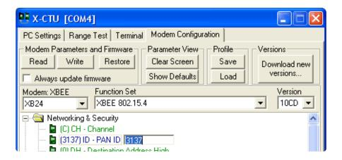
If you are using a terminal to connect, use the ATID command to set and check the PAN ID
