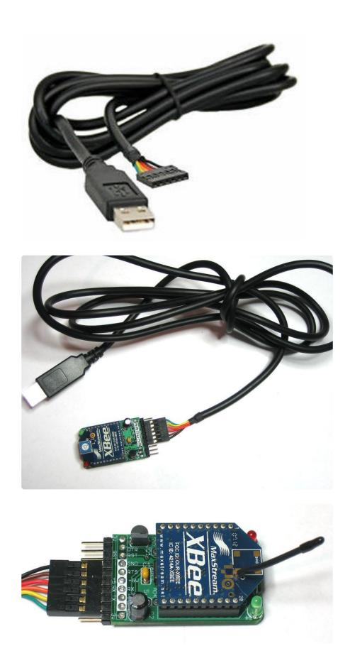
Another method of connecting is using a USB or serial breakout board. Each breakout board is going to be a little different so check the documentation. Make sure the transmit/receive pins are not swapped, etc.
