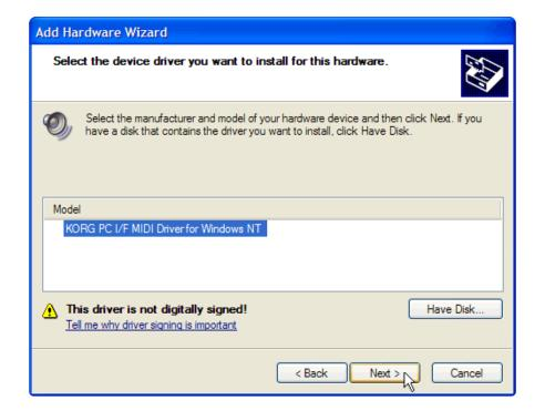
Make sure the FTDI cable is set to COM2, 3 or 4 because the driver can't cope with higher numbers. You can set the FTDI cable's COM port in the Device Manager. Set the KORG driver to the correct COM port.
