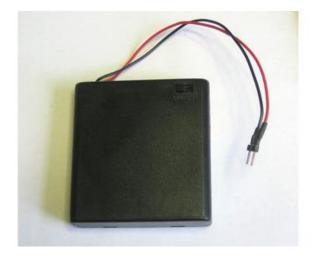
Get the 4xAA battery holder setup. Solder the red and black wires to a double-header. This will make it easy to plug into the breadboard. I used some heatshrink to keep the two from touching. It's easier if you place the header in the breadboard while soldering.
