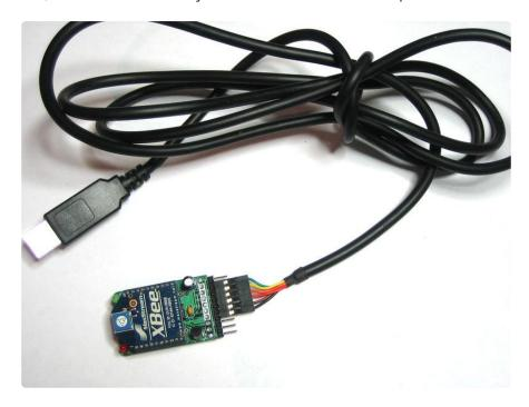
This XBee should also be firmware updated but it doesn't have to be set to 31250 baud! That's because the XBee transmits wireless data in its own ZigBee protocol, not plain serial. You can have one XBee communicating at 31,250 baud and another at 9600 baud and they'll pass data back and forth just fine. Anyways. Connect up to XBee using X-CTU or use another terminal. I suggest a terminal program that lets you see hex values for transmitted data which is why X-CTU is pretty rad.
