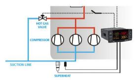
To detect the suction superheat an auxiliary probe among P4 (term. 3-13) has to be set as superheat temperature probe.
