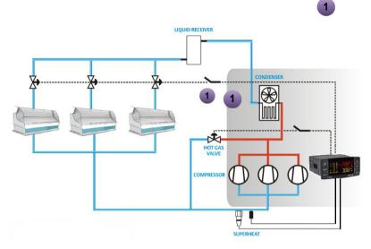
To enable this function set one relay by the parameters **oA2** or **oA3** or **oA4** or **oA5**, as flood protection, El **oA4 = Liq**, and then connect it to the external device that blocks the cabinet injection. NOTE: the relay set as flood protection is automatically activated even when the controller is in stand-by mode.
