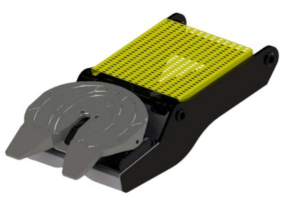
The XE20 power steering and 5th wheel boom lift are operated hydraulically and powered by a hydrostatic pump.
