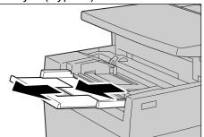
**NOTE:** If necessary, extend the extension flap. The extension flap can be extended in two stages. When pulling out the extension flap, do it gently.
