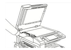
2. Use a lint-free cloth and Xerox<sup>®</sup> Cleaning Fluid to clean the underside of the document cover and the document feeder.
