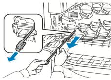
5. Slowly push the LED printhead cleaner back into the printhead until it stops.
