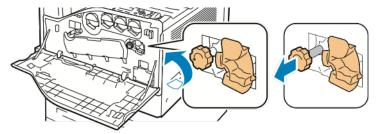
4. Pull the transfer belt cleaner straight out of the printer.
