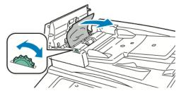
4. If the message instructs you to open the inner cover, lift the lever with the green tab to open the inner cover.
