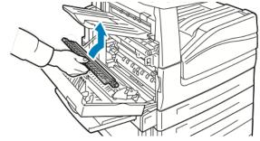
7. Place the used transfer roller in the plastic bag.
