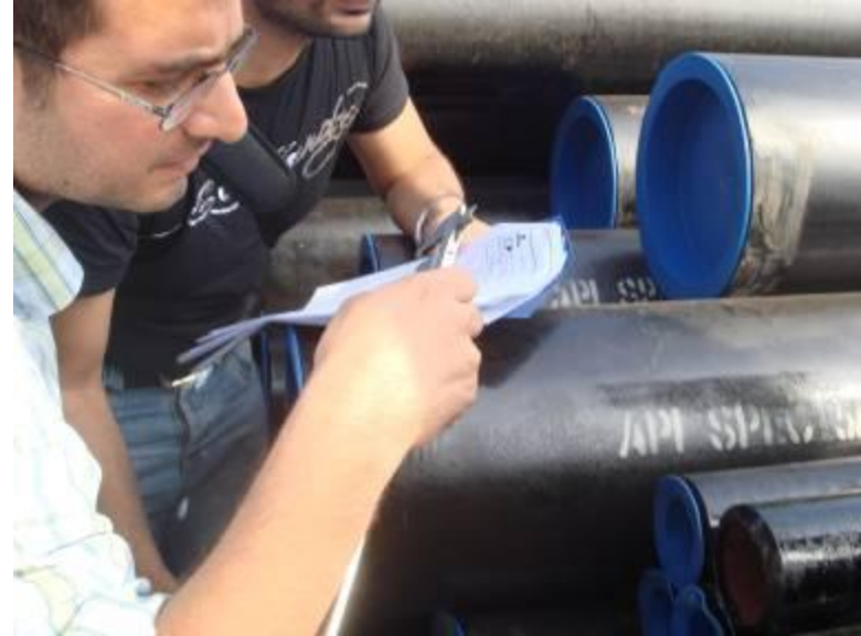
Customer check the pipe dimension
