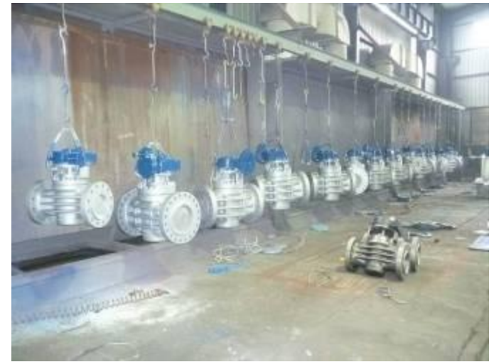
Plug Valve under the painting process
