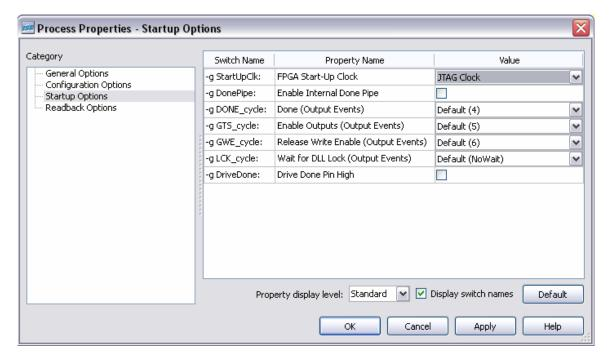
After selecting the appropriate start-up clock value, click OK and run the Generate Programming File process. After this process completes, a configuration .bit file should appear in the directory where your project is located.
