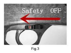
To remove the safety to "OFF", move safety button to have "F" seen. In this position, the gun is ready to shoot. (Fig.3)
