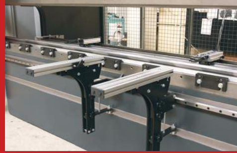
Two front linear guided sheet supports
