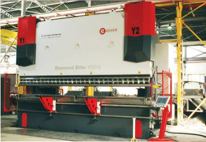
Elite 1000-60 (1100 ton x 20 feet) with 6 axis back gauge
