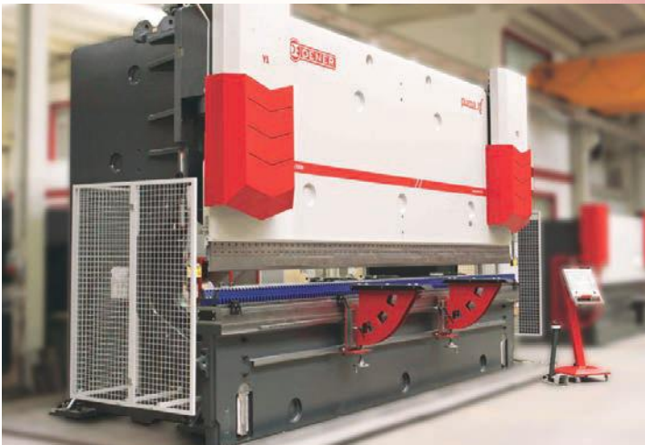
Elite 1000-70 (1100 ton x 23 feet) with Adjustable v Die
