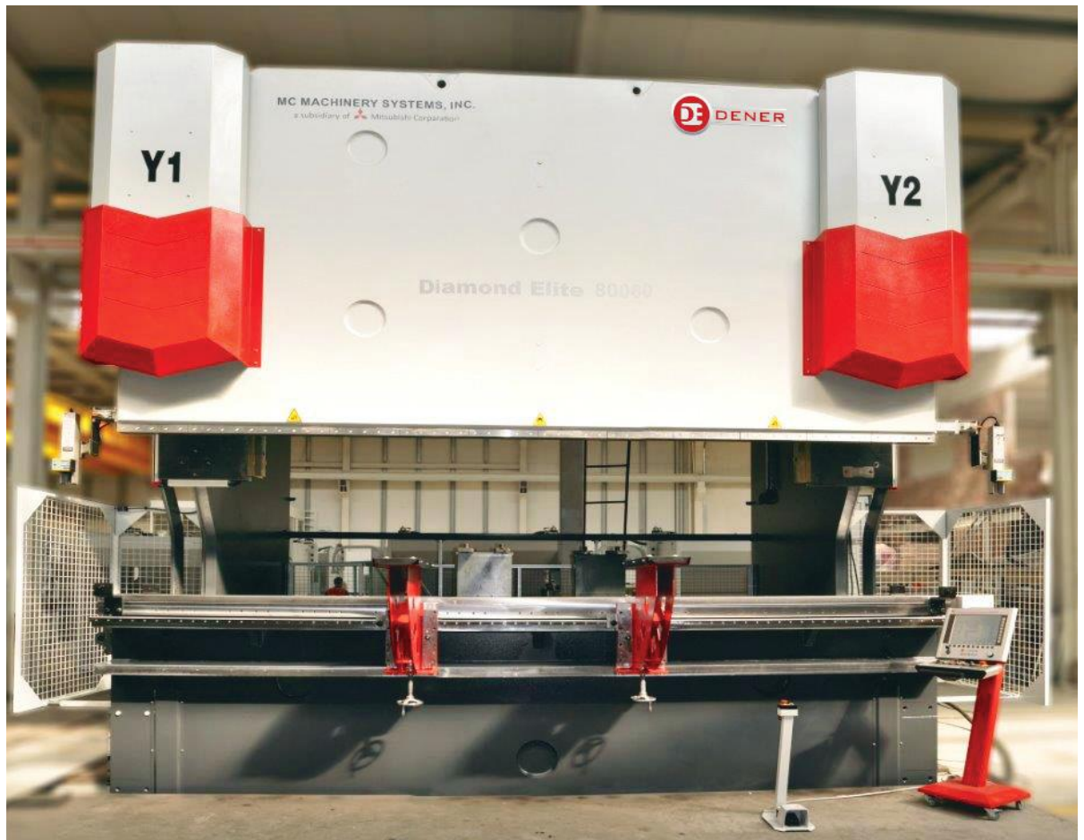
Elite 800-60 (880 ton x 20 feet) with 6 axis ATF back gauge & 40" ram stroke
