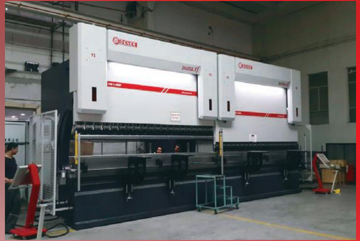
Tandem Elite 500-40 (550 ton x 13 feet) (1100 ton x 26 feet tandem)
