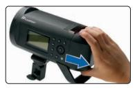
1. To release the battery, first turn off the power.
