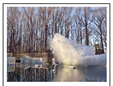
After six months of testing different water landing scenarios, an 18,000 pound Orion mockup took its final splash into the LaRC Hydro Impact Basin on January 6, 2012. This test represented a worst case landing for an abort scenario in rough seas. This scenario is not likely to occur during actual vehicle operation, but is essential for the validation of analytical models. As was the case with Apollo, the Orion MPCV flight design will feature an onboard up-righting system.
