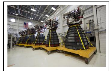
In October 2011, all fifteen Space Shuttle Main Engines are together for the first time inside NASA's Engine Shop at KSC. They will be prepped for shipment to SSC where they'll become part of the propulsion used on the SLS. Each engine is capable of generating a force of nearly 400,000 pounds of thrust at liftoff, and consumes 350 gallons of fuel per second. They are engineered to burn liquid hydrogen and liquid oxygen, creating exhaust composed primarily of water vapor.
