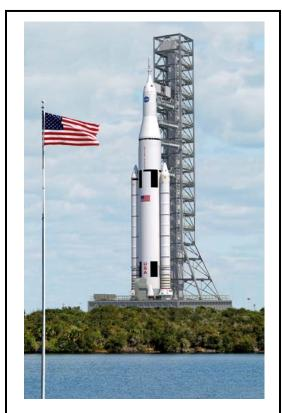
An artist's conception shows the SLS ready to launch. The SLS will eventually have a lift capacity between 70 and 130 metric tons, but not every mission will require that much lift. The SLS modular architecture allows use of different core stage, upper stage, and first-stage booster combinations to match the mission requirements.
