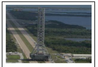
The mobile launch tower that will support NASA's next exploration rocket is on the crawler-transporter to launch pad 39B at KSC. The 6.8-million pound launcher, towering some 400 feet off the ground is making the 4.2-mile trip to give engineers data on how much the tower sways and wiggles during the journey. Then two weeks of tests at the pad will provide a comprehensive "fit check" to test clearances and connections.
