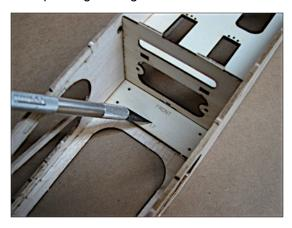
Bond cross-grain doublers F10b within fuselage assembly as illustrated.
