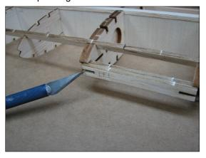
Use plan sheet as a guide to locate and install X rib trussing in leading edge of wing. Trussing fits between top and bottom spar, against spar web, and centered with leading edge notch in rib/sub-rib. Tack glue to retain.
