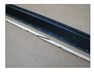
Fit W1 to forward most notch in ribs spanning left and right ribs R5. Tip: Invert wing and use a gentle rocking motion against a hard flat surface to seat W1.
