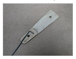
Using thick CA glue, laminate F14c on top of F14b.
