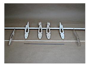
Carbon fits into recess cut into S1 lower spar jig and spans between R2 ribs across center of wing section.
