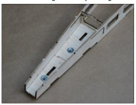
Invert fuselage and install F12 to underside of F11.
