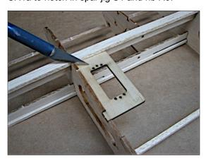
Using thick CA, laminate SR1b balsa doubler to top of SR1a.
