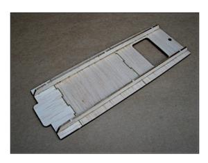
Using thick CA glue, bond H1 on top of H2 using tabs from H1d to locate H1 atop H2.
