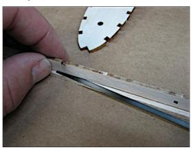
Carbon is captured by S1 jig and R1/R2 ribs.
