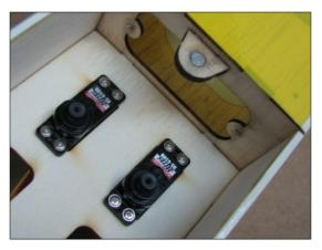
Use radio, or servo tester, to electronically center servos. Install control horns to servos then pass pushrods through housing from tail of aircraft ending through E/Z connector as illustrated below.
