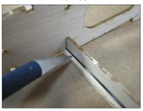
Flatten wing against work surface, inspect all parts to ensure proper fit, then tack glue assembly together where ribs meet trailing edge and lower spar assembly.
