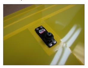
Aileron servo wire should pass through opening in W6 at bottom of wing.
