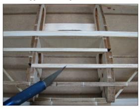
Fit remainder of turbulator stock for both top and bottom of wing. Remember turbulators sit 3/32 in proud of interior ribs and flush with ribs R1 and R5. Flatten wing against your building surface then glue turbulator stock at each contact point with ribs.
