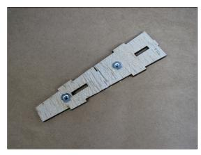
Study photo below then install F11 and F6 together between fuselage sides at tail. Note that the flange of installed blind nuts must face inside fuselage assembly. Tack glue.
