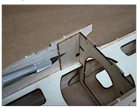
Assemble the top (F7) and bottom (F8) fuselage formers from sub-assemblies F7a/ F7b and F8a/F8b respectively.
