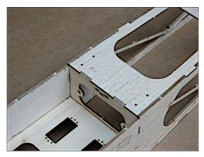
Bond the of plywood hardpoint F17 with "FRONT" flush against aft side of former F3 and spanning fuselage sides.
