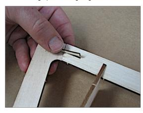
Create and install sub spar. Use a scarf joint to join together two 1/8 in. x 3/16 in. x 24 in. balsa sticks. Cut joined sticks to 43 in. length and install spanning wing assembly. Note that sub spar will seat against notch in wing wing tip as indicated below.
