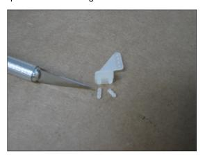
Install control horn to laser drilled holes on push-rod side of elevator and rudder and bond with medium CA glue.
