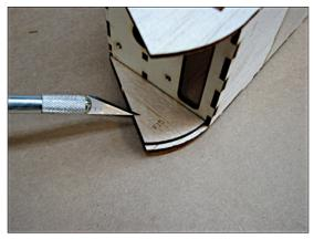
Install F16 between fuselage sides forward of F1 and along lower edge of F15.
