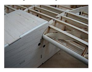
Use sanding block to taper SR1b to match rib.
