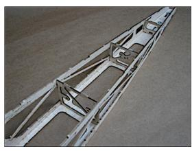
Install optional servo pocket ply doublers F3 to right and left side of fuselage forward of F6.
