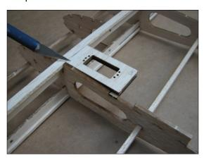
Using thick CA glue, laminate W4 to recess in T1 at wing trailing edge.
