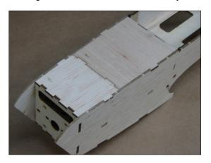
Glue G2 into position spanning fuselage sides as indicated below.
