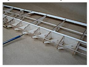
Cut 1/4 in. square stock to fit leading edge and bond to wing using medium CA glue.
