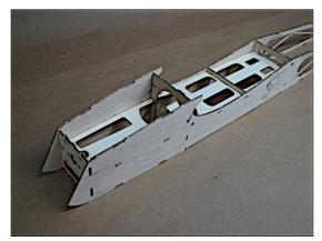
Using thick CA glue, install the cross-grain doubler F10a forward of former F2. (F10a fits flush against F2 and F0 center crutch)
