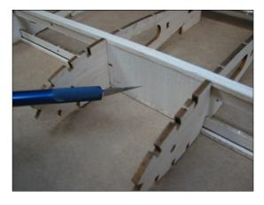
Align R1a with notches in R1 then use thick CA glue to laminate R1a to inside surface of ribs R1.
