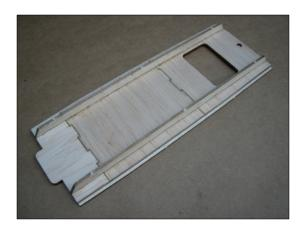
Glue one 3/16 in. diameter magnet within locating hole in H1.
