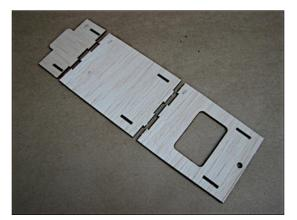
Dry fit H1d doublers to right and left side of H1 hatch assembly. The tabs in H1d should extend proud of underside of H1d by 1/16 in.
