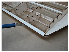
Dry fit 1/8 in. x 3/16 in. x 24 in. turbulator stock staggered at wing center as illustrated.
