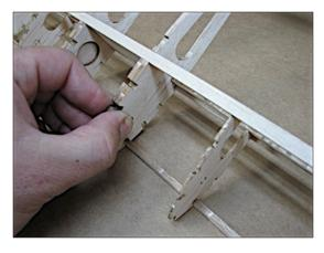
W1 fits flush with ribs R1 and R5 but sits 3/32 proud of the top surface of ribs R2-R4 and all sub ribs SR.
