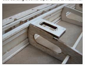
Carefully remove material. Tip: protect surrounding spar and ribs from sanding block action with masking tape.
