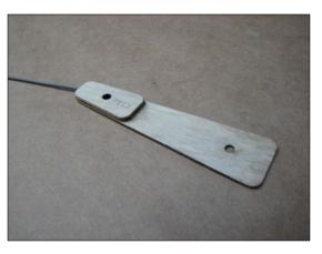
Once glue has cured, straighten wire where it exits plywood then bend down at 45 degree angle (use plan set to gauge bend and angle) complete tail skid by making an upward "U" shape bend at end of skid.
