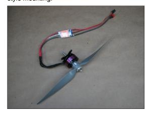
Using provided 4-40 x 3/8 in. steel machine screws secure motor to firewall. Tip: Shim left side of motor mount with 1/16 plywood washers (located on sheet 18/19) for right thrust.
