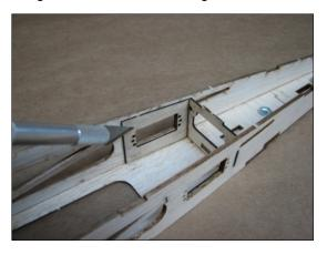
Complete fuselage assembly by installing former F9 spanning fuselage sides and F3. Now, square fuselage to worktable and bond all joints with thin CA glue.
