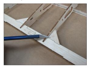
Fit S2 upper spar jig to wing assembly.
