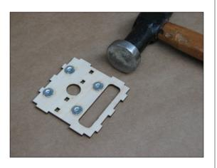
Key F1 firewall to the front of F0 center crutch, with flange portion of blind nut facing aft.
