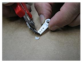
☐ Install Du-Bro RC Mini E/Z connector provided with your pushrod kit (DUB922) to inside hole of trimmed servo arms.
