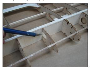
Using thick CA glue, laminate together both LE1 center section leading edge parts, then install spanning ribs R1.
