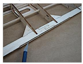
Fit and tack glue all SW2 vertical grain shear webbing in-between ribs and sub ribs spanning R1 through R4. Webbing is notched on one side where it partially extends into lightening hole gap at each sub rib SR.
