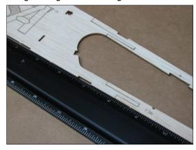
With straight edge providing an alignment aide, install trussed components within fuselage side, matching A to A and B to B.
