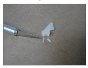
Install control horn to laser drilled holes on servo side of ailerons and bond with medium CA glue.
