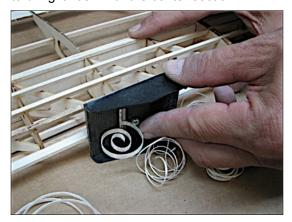
Use a long sanding bar loaded with 250 and 400 grit paper to round out leading edge to match wing saddle of fuselage.
