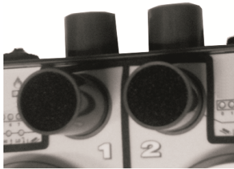
Figure 3-4: Filter at inlet of system
