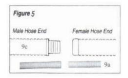
One of the hose sections has 2 female ends and a hose protector. This section should be fitted last and attached to the pool's vacuum connection.
