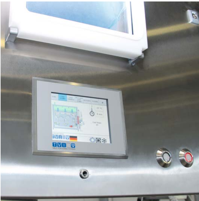
The portioning system (above) is operated via a customer-specific CP6901 12-inch Control Panel. The shock freezer (below) is operated via a built-in CP6907 Control Panel with a 5.7-inch screen..
