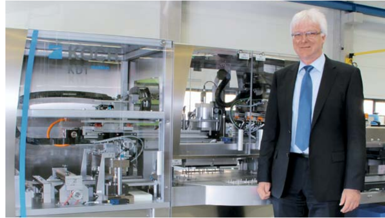
Jürgen Welker, Head of the Automation and Service Division at KOCH, in front of the new KDT medplus rotary table machine, which is conceived for cleanroom use in medical fields.
