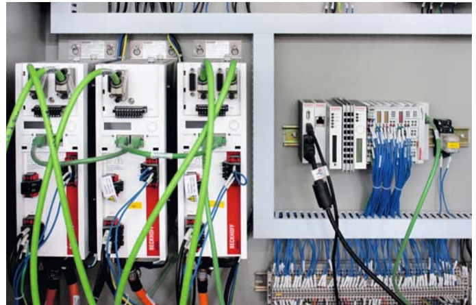
AX5000 series EtherCAT Servo Drives are used for exact positioning of the motors. The axis positions are sampled in real-time via the measuring probe functions of the AX5000 Servo Drives.
