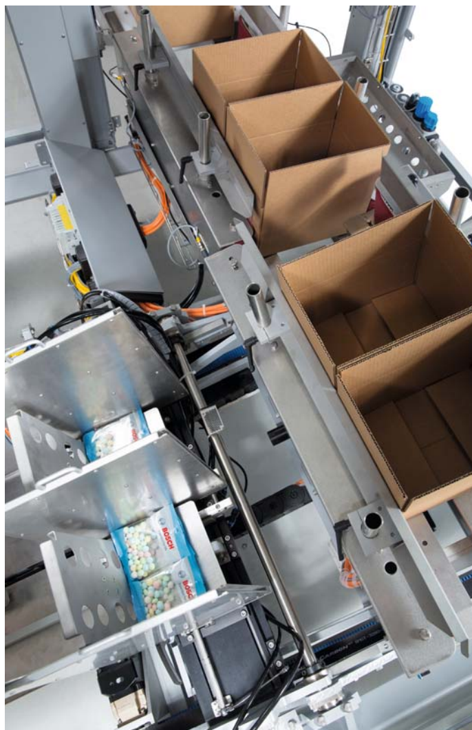
Capable of picking and placing up to 180 bags per minute, the Bosch CCM 3100 machine's single frame is attached to an infeed system that accepts products from VFFS and HFFS primary packaging machines
