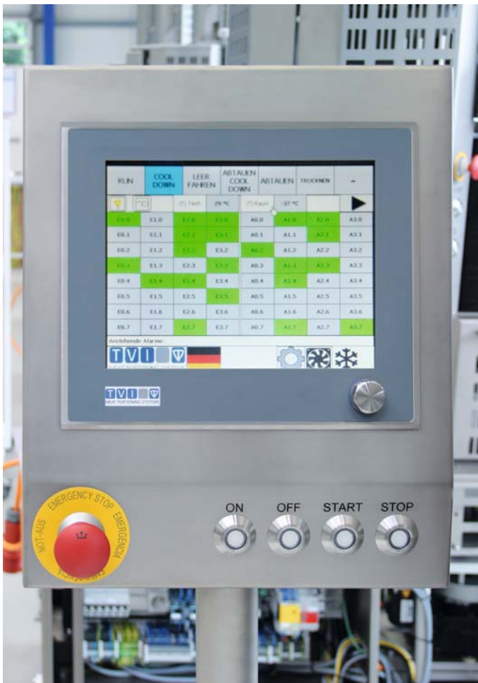
The portioning system (above) is operated via a customer-specific CP6901 12-inch Control Panel. The shock freezer (below) is operated via a built-in CP6907 Control Panel with a 5.7-inch screen..
