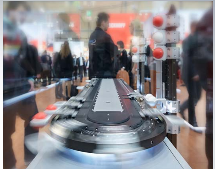
Figure 7: The combination of a horizontal XTS and vertical systems – here a demo application from the 2014 Hannover Messe – is a great way to separate specific elements from the product stream and rearrange the stream in accordance with the desired criteria.
