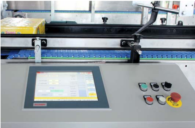
The shrink film packaging system is operated via a built-in "Economy"-type Control Panel.
