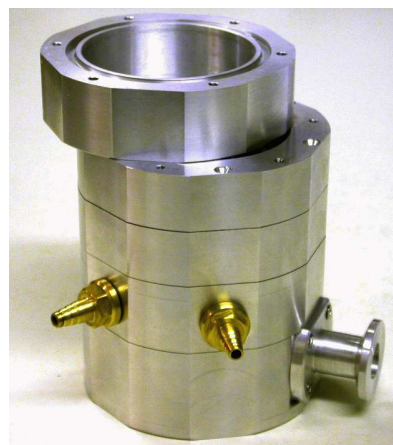
Figure 4: CCD camera head. \phi=9 cm; height=12cm.
