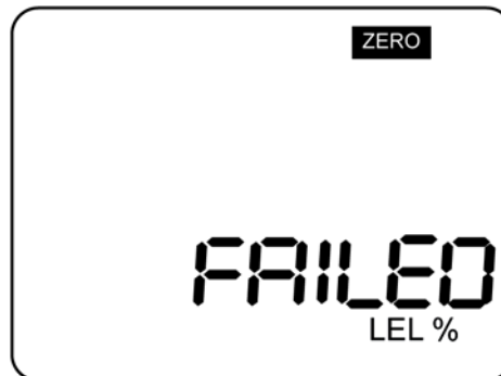
Figure 27 Zero Calibration Display - Failed
