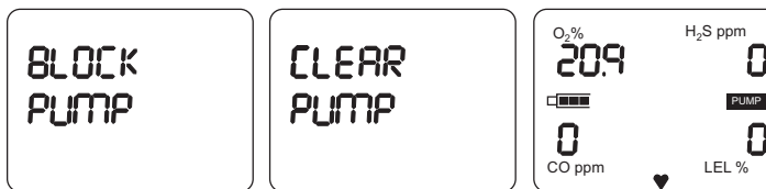
Figure 16 Pump Displays - Start Up
