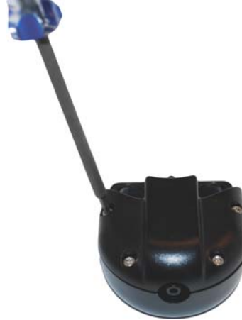
Figure 34 Removing Pump Screws
