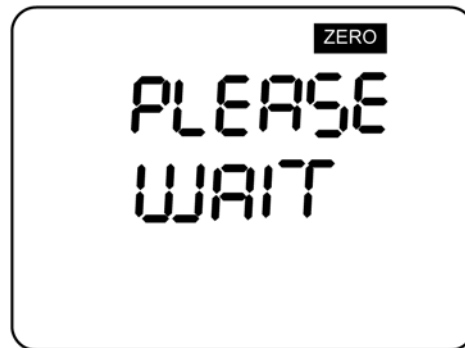
Figure 25 Zero Calibration Display - In Progress
