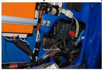
H. Zip tie supplied harness into place along the factory harness inside the door.
