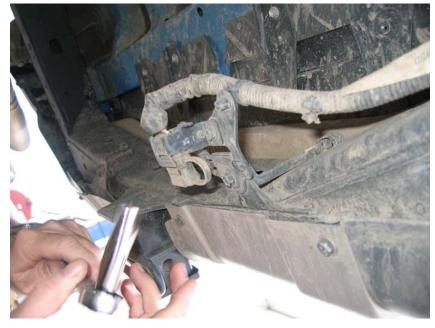
H. Remove the plastic bumper trim by prying outward and rearward simultaneously on the plastic corner protectors thereby freeing the plastic shell, set aside as it will not be reused.
