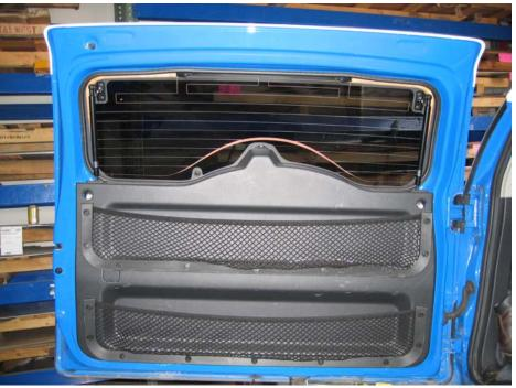
B. By hand GENTLY pull the panel away from the rear door. Open the rear door window to release the panel at the top. See Image Below.
