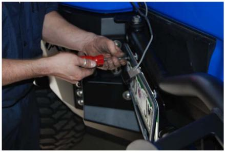
*N.* Use Zip Ties to secure the harness to the tire carrier and over to the pivot. Be careful to route it in a way that allows the tire carrier and the rear door to operate independently of each other without damaging the harness.
