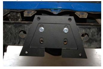
G. Using two people (One on each Corner Wing), with one more to be free to install bolts, lift the bumper into place. Be extremely cautious as to not scratch the paint with the Corner Wings. The third person can now install the four supplied metric bolts into the bottom of the frame through the Fab Fours Frame Mount Brackets. Do not fully tighten these at this time. See Image Below.
