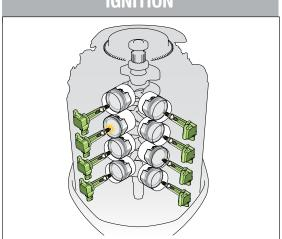
Advanced engineering features include spark plug caps with the ignition coils built right in. The result is increased performance and reliability in a much simpler and more compact design.
