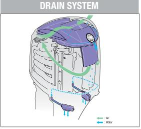
The F350C employs a new cowling drain system to easily and efficiently drain away water that enters the cowling during normal engine operation. Incoming air is routed through a labyrinth of passages that trap and drain water before it enters the engine's intake, for enhanced reliability.
