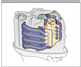
All air entering the F350C is routed through a single 81mm intake that is controlled by the ECM to ensure the precise amount of air necessary for any given condition. This helps maintain optimum power and efficiency.
