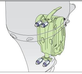
The F350C features four motor mounts made of strong forged aluminum, which means they're compressed in molds for much greater strength than cast aluminumtype mounts. The oversized mounting bracket features the same bolt pattern and centerline as the F250, but uses two additional mounting bolts for a total of six (not visible in this rendering). It is designed to handle the engine's power while minimizing noise and vibration.
