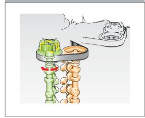
This system advances and retards the angle of the intake camshaft to dramatically increase power and throttle response in the low- and mid-rpm ranges. This gives the engine substantially greater torque between 2000 and 3500 RPM to plane large offshore boats with authority.
