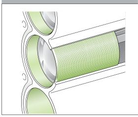
The outer cylinder sleeves of the F350C feature a "dimpled" surface. This helps maintain the roundness of the cylinder for decreased oil consumption, and increase the cooling surface area of each cylinder for added reliability.
