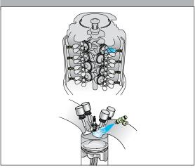
Seven different sensors constantly measure vital atmospheric conditions and engine functions to give the Engine Control Module (ECM) the information needed to precisely and instantly adjust the fuel/air mixture for optimum performance and economy.
