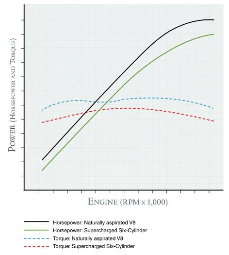
Technically, torque is twisting force. It is a measure of work, while horsepower is a measure of work over time. Torque is what you feel when you open the throttle and your boat leaps to plane. Torque *is* what matters.
