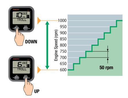
Controlled by optional Helm Master® or the Command Link®/Command Link Plus® tachometer, the operator can adjust the engine's trolling speed from 600 to 1,000 rpm in 50 rpm increments, which helps to provide precise and consistent trolling speeds in an array of conditions.
