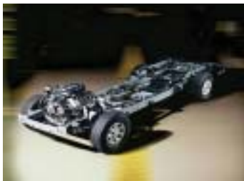
Titan's newly designed body-on-frame platform
