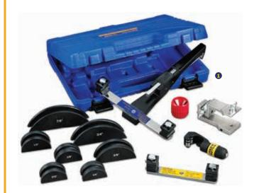
Easy one hand bending of 1/4" to 7/8" soft copper and soft aluminum. Hard copper must be annealed before bending.
