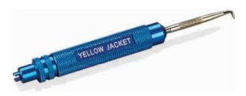
Easily remove worn gaskets from hoses and replace with new gaskets. Sharp, angled pick is long enough to pull the gasket from the gasket cup. Notch on the opposite end of the pick for placing the depressor inside the hose. For protection and safety, pick stores inside case along with five replacement gaskets (included).
