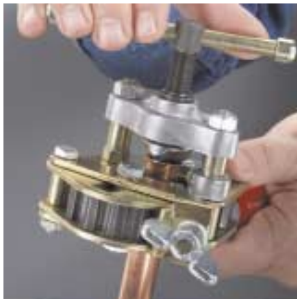
Deluxe 45° Flaring Tool – The only full range 1/8" to 3/4" O. D. flaring tool available for soft copper, brass, and aluminum tubing (Page 102).
