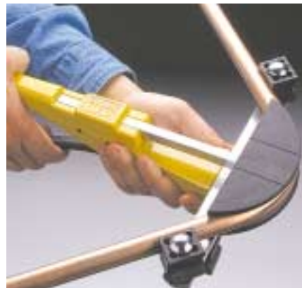
Ratchet Hand Bender – Versatile, easy-to-use bender for soft copper, aluminum and light wall hydraulic tubing (Page 107).
