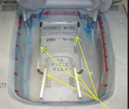
Trench with Magnets
