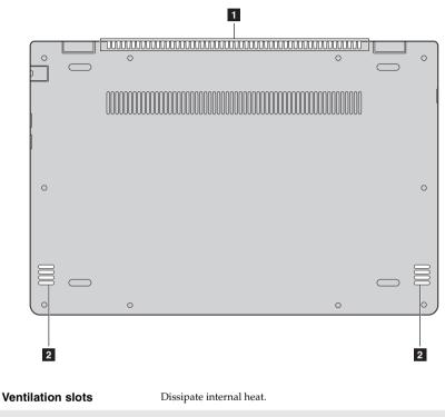
Note: Make sure that the ventilation slots are not blocked or else the computer may overheat.
