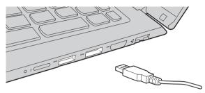
The first time you plug a USB device into a particular USB port on your computer, Windows automatically installs a driver for that device. After the driver has been installed, you can disconnect and reconnect the device without performing any additional steps.
